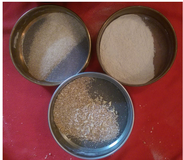
Fig. 2 Experimental flour types: fine ( <0.5 mm), coarse grain or fine bulgur ( >0.5 mm) and coarse bulgur ( >1 mm) mixed with cracked grain and flakes
