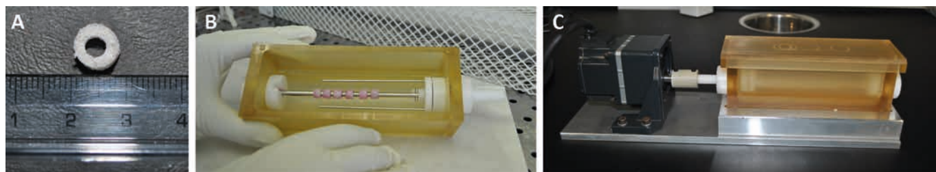
Fig. 3 - (A) Polyurethane foam (PUF) cylindrical sample, (B) PUF scaffolds located on a plain stainless steel mandrel in the InBreath bioreactor (8). (C) Bioreactor setup used for the different configuration culture systems as it is inserted in the incubator; in this picture the Petri dish-like cap, which allows for oxygen exchange with the controlled environment of the incubator while maintaining sterility of the inner chamber, is visible.
