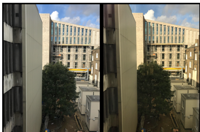
Figure 6. Evaluation of visible transmittance through a typical VO 2 film (sample B, thickness 72 nm) deposited on glass showing the outside view. The photographs of the outside view were taken without (left) and with (right) the VO 2 coating. Photograph courtesy of Delphine Malarde. Copyright 2016.
