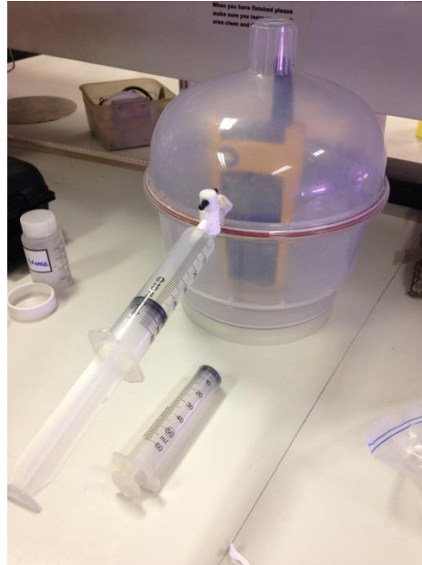
Figure V.5. Sealable vessel for the measurement of the highest CO 2 concentration used in the preliminary experiments.
