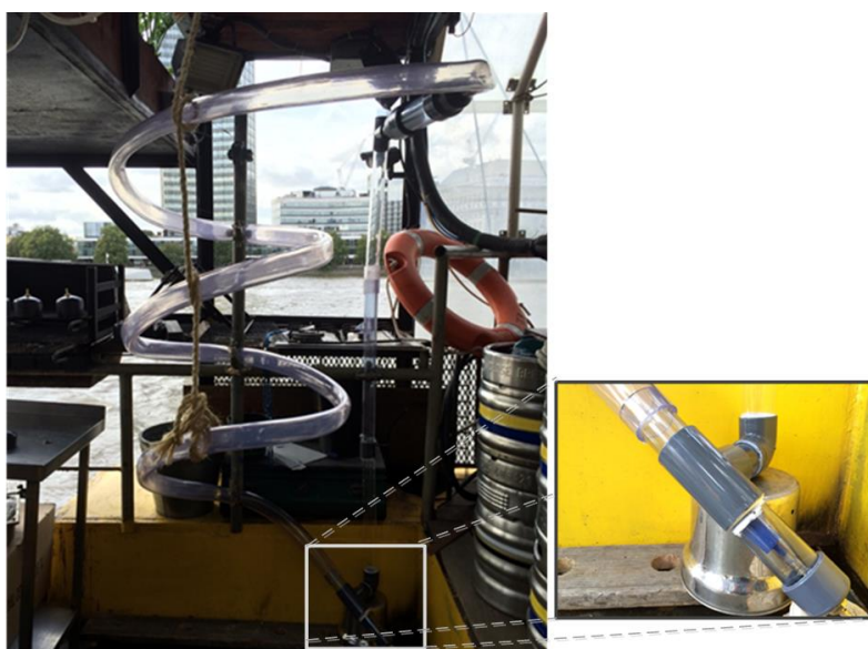
Figure III.2. Side view of the hybrid helical airlift photobioreactor constructed onboard Tamesis (left picture) and its bottom connection (right picture).
