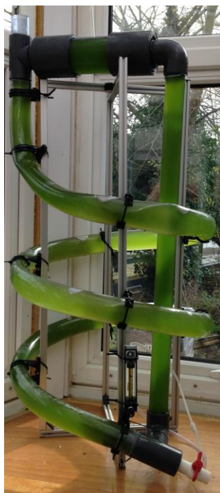
Figure III.1. Side view of the hybrid helical airlift photobioreactor constructed at the Camley Street Park.
