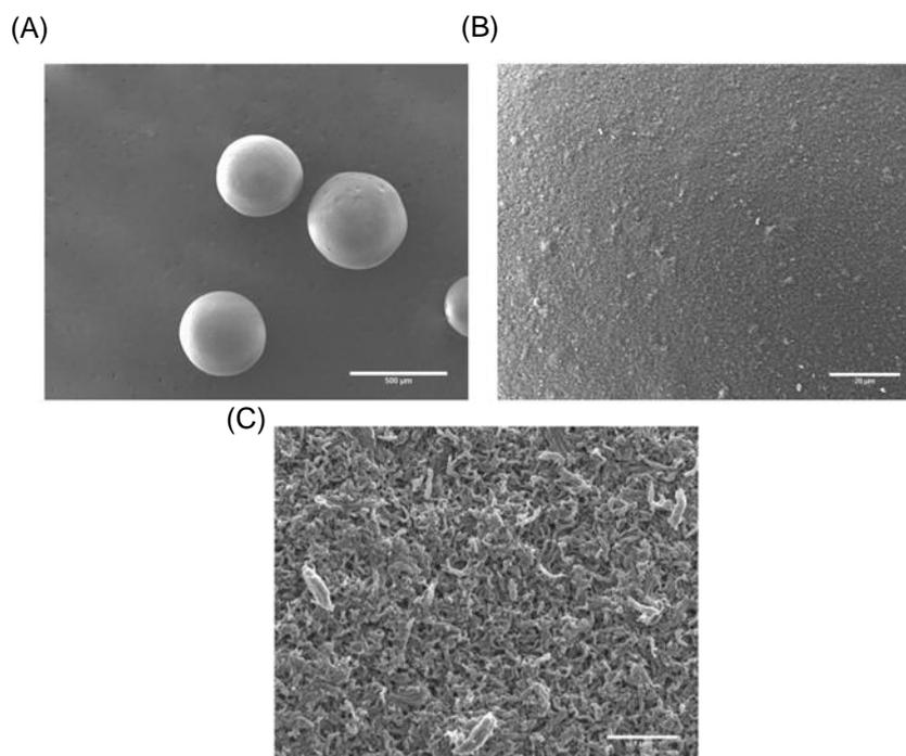
**Figure 5.11** EM of SpheriTech beads at (A) x1000, (B) x10,000 and (C) x20,000 magnifications. Scale bars are 500μm, 20μm and 1μm.
