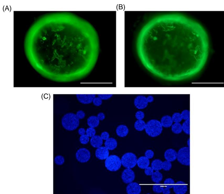
**Figure 5.19** SpheriTech bead autofluorescence. (A-B) 470nm excitation and 525nm emission; (C) 360nm excitation and 447nm emission. Scale bar = (A-B) 250  $\mu\text{m}$  or (C) 1000  $\mu\text{m}$ .
