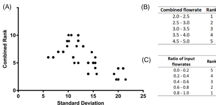
**Figure 5.9** Impact of flowrates upon bead heterogeneity. By grouping combined flowrates and flowrate ratios tested into 5 tiers, a rank could be applied to every condition tested. A high rank related to smaller beads and a low rank to larger beads. The 5 ranks for (B) combined flowrate
