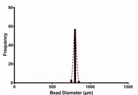
**Figure 5.5** Particle size distribution of SpheriTech beads manufactured in a microfluidic droplet generator at 1 μl/s aqueous phase and 3 μl/s solvent inputs (N=84).
