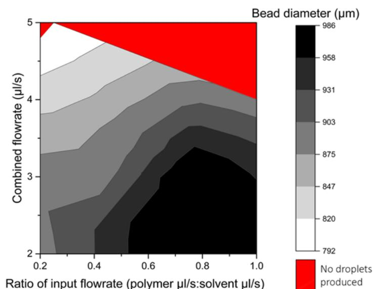
**Figure 5.8** Analysis of bead size from different manufacture conditions. By varying the ratio of the polymer:solvent phase between 0.2 and 1, and combined flowrate between 2 $\mu\text{l/s}$  and 5 $\mu\text{l/s}$ , the size of beads produced was measured and plotted on a contour plot. The area shaded in red is where no beads were formed due to agglomeration of droplets in the T-junction.
