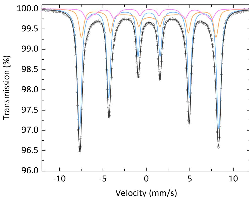
**Figure 5.16** Mössbauer spectrum of Alfa Aesar iron oxide. An  $^{57}\text{Fe}$  radioactive source was oscillated by  $\pm 15\text{mm/s}$  at room temperature next to a sample of dried SpheriTech beads and the absorption (%transition through the sample) recorded for  $N=3$  samples. Experimental data points are shown as circular dots ( $\circ$ ), the fitted spectrum is the dark black line, the sub-spectra are the coloured lines.
