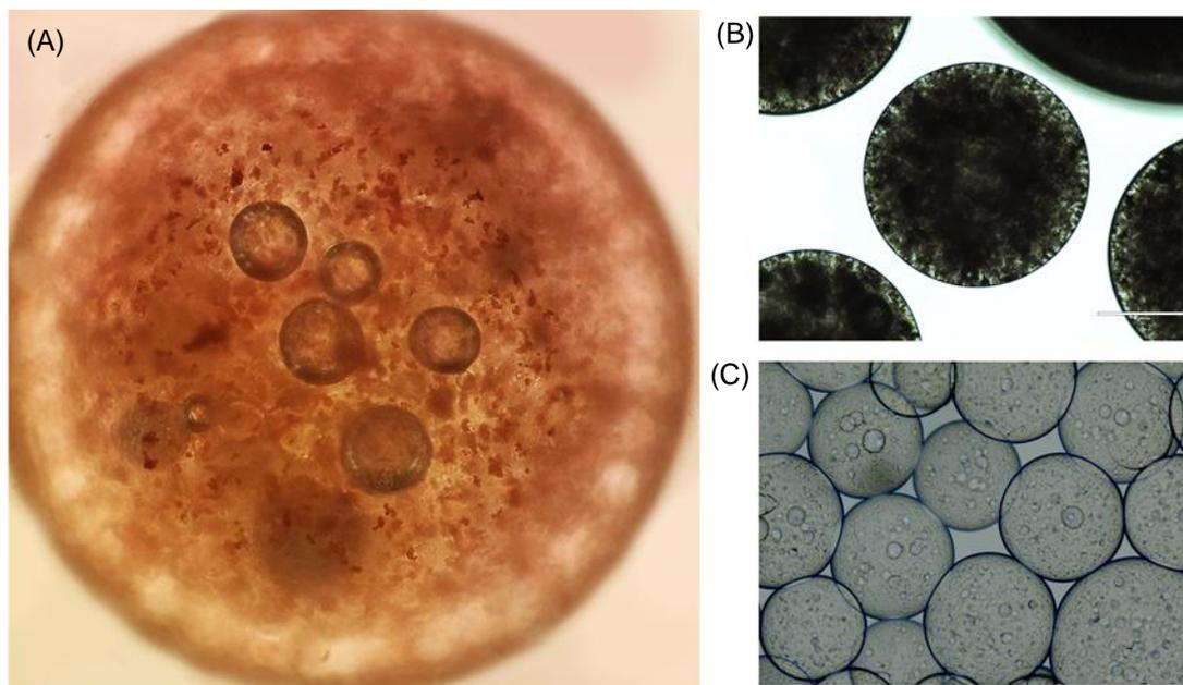
**Figure 5.1** Microscopy images of SpheriTech beads. (A) Bead with 1g iron oxide and hollow microballoons; (B) Beads with 2g iron oxide only; (C) Beads with hollow microballoons only.
