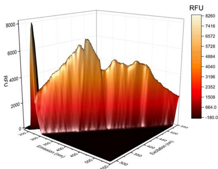
**Figure 5.20** Autofluorescence of SpheriTech beads. Fluorescence intensity was measured over across a range of 230-550nm excitation and 280-550 nm emission wavelengths with a step size of 2nm with SpheriTech beads in PBS. A RFU of 0 to 8200 was measured.
