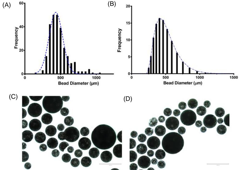
**Figure 5.3** Frequency particle size distributions of SpheriTech beads manufactured in a reactor. (A) Microscopy ( $N=268$  beads) and a (B) particle size analyser ( $N=3$  runs) was used to measure particle size. Phase contrast images of beads used in the (C) microscopy and (D) particle size analyser were taken. Scale bar =  $1000\ \mu\text{m}$ .
