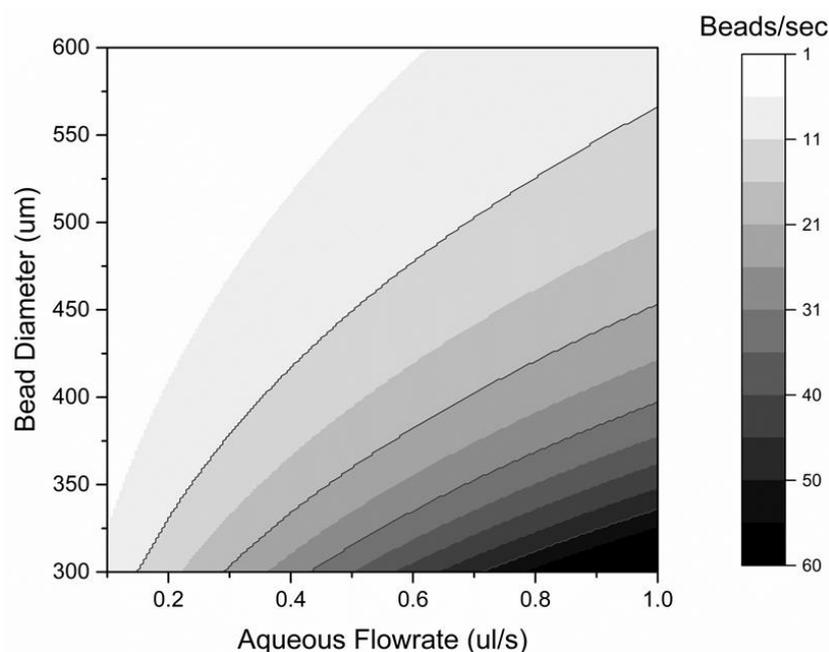
**Figure 5.10** Production rates of beads using the microfluidic chip. At a range of aqueous flowrates between 0.1  $\mu\text{l/s}$  and 1  $\mu\text{l/s}$ , a contour plot illustrating the amount of droplets generated per second to produce different bead diameters is shown using a scale from 1-60 beads per second.
