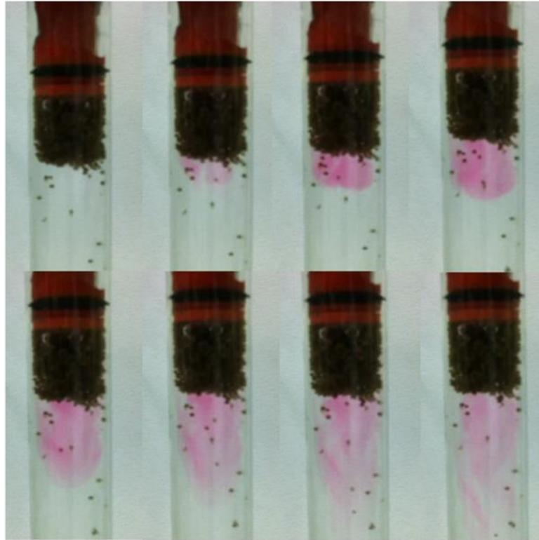
**Figure 5.17** Visualisation of buoyant beads under flow. SpheriTech beads forming a floating inverted expanded bed in a 1cm diameter chromatography column under downwards flowrate against gravity. A pink dye was injected into the PBS to visualise flow. Each image is 0.5 seconds apart.
