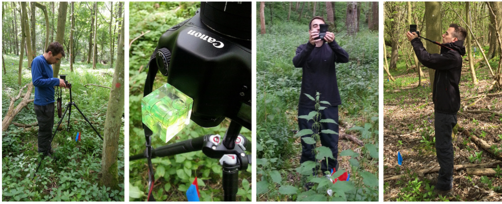
Fig. 2. User setting up a tripod levelled DHP (far left – compass positioned over camera lens) with bubble level attachment (middle left) and using the hand-leveling approach (middle and far right).
