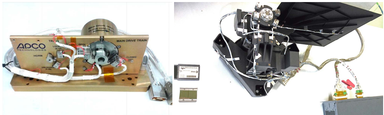
Figure 9: (left) The EM for the Shutter. (right) The STM for the shutter. The shutter leaf is at the top of the image, and covers the full CCD focal plane. The mounting structure is in the centre.
