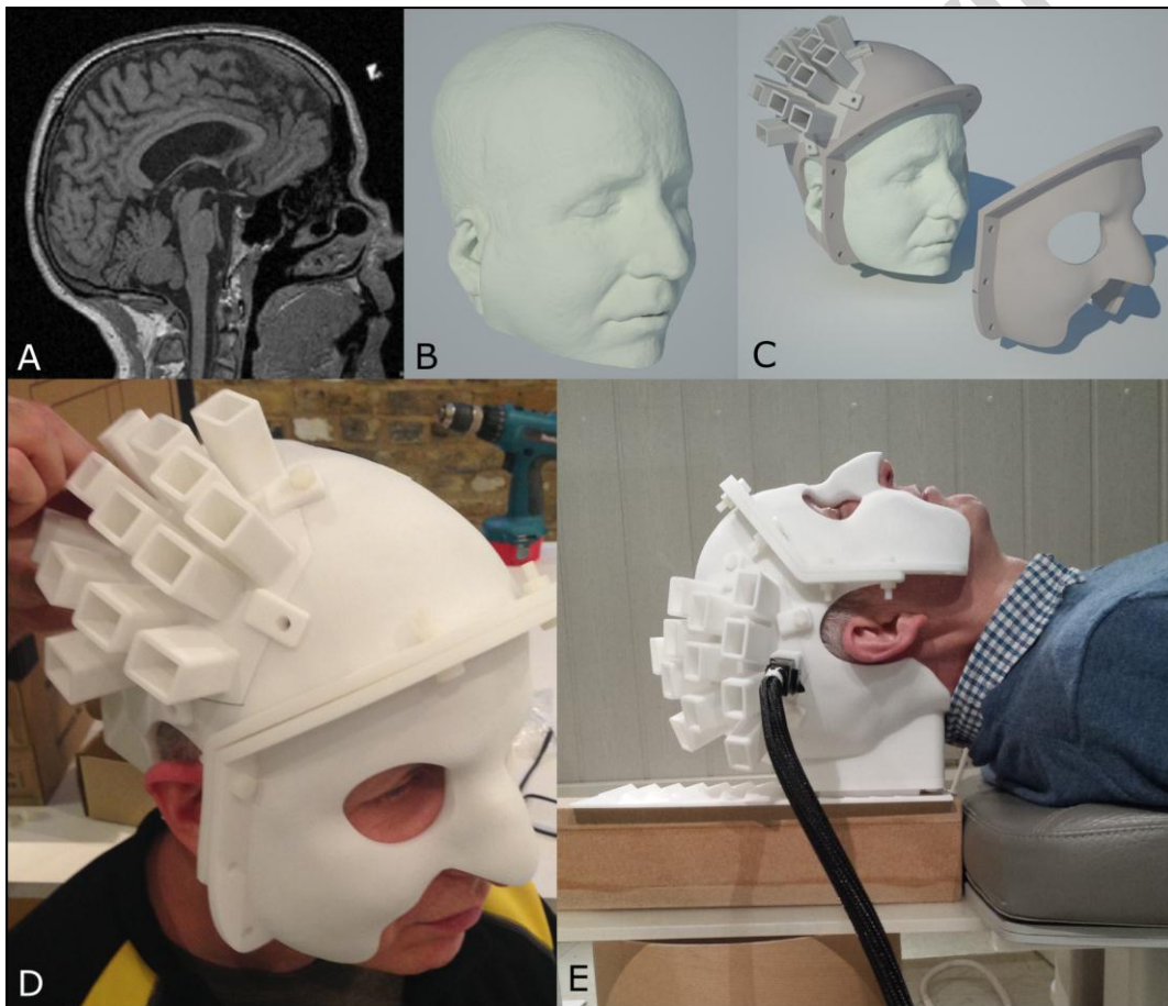
Figure 2: Head-cast design and fabrication: A) Single sagittal slice from the anatomical MRI. B) Outer head surface extracted from MRI. C) CAD model of the head-cast with slots designed to house the OPM sensors over sensorimotor cortex. Slot positions are based on a-priori prediction of the spatial topography of scalp field pattern, derived from previous SQUID measurements in the same subject. D) 3D-printed head-cast on subject. E) Subject in situ with the OPM attached. Note that the head-cast is not only fixed rigidly to the subject's scalp, but is also fixed relative to the shielded room, thus eliminating any sensor motion relative to the subject, and subject motion relative to the MSR.
