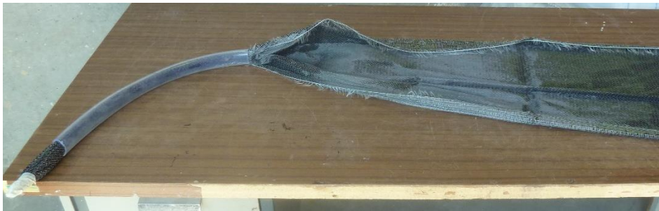
Fig. 3. FRP “strand”: rolled FRP sheet passed through plastic tube
