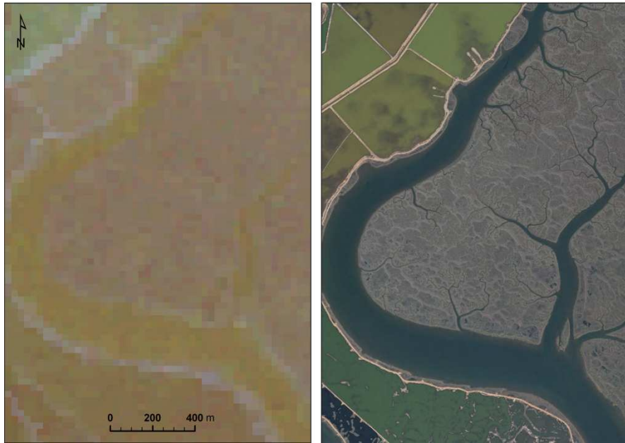
Figure 1.11 Illustrative sample of 30m spatial resolution Landsat-5 image (on the left) and 1m spatial resolution aerial photograph (right) for a saltmarsh.
