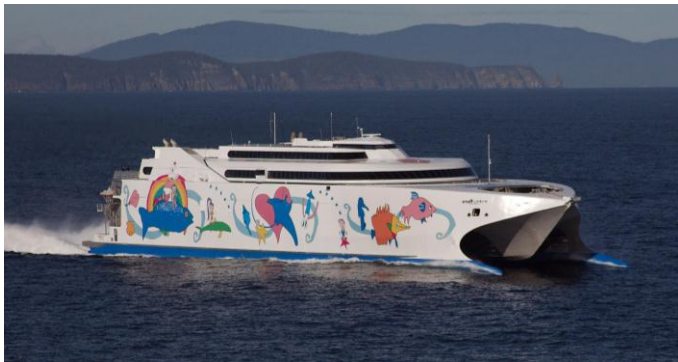
Fig. 1. INCAT Tasmania hull 064 – Nachan Rera. A 112m wave piercing catamaran.
