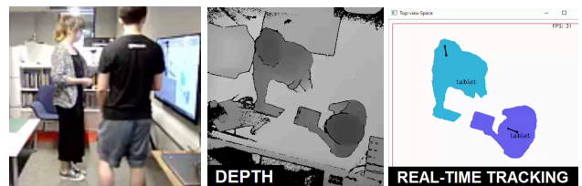
Figure 12. Recognizing two people and their devices when in front of large screen (left to right: space, depth image, real-time tracking of EagleSense ).
