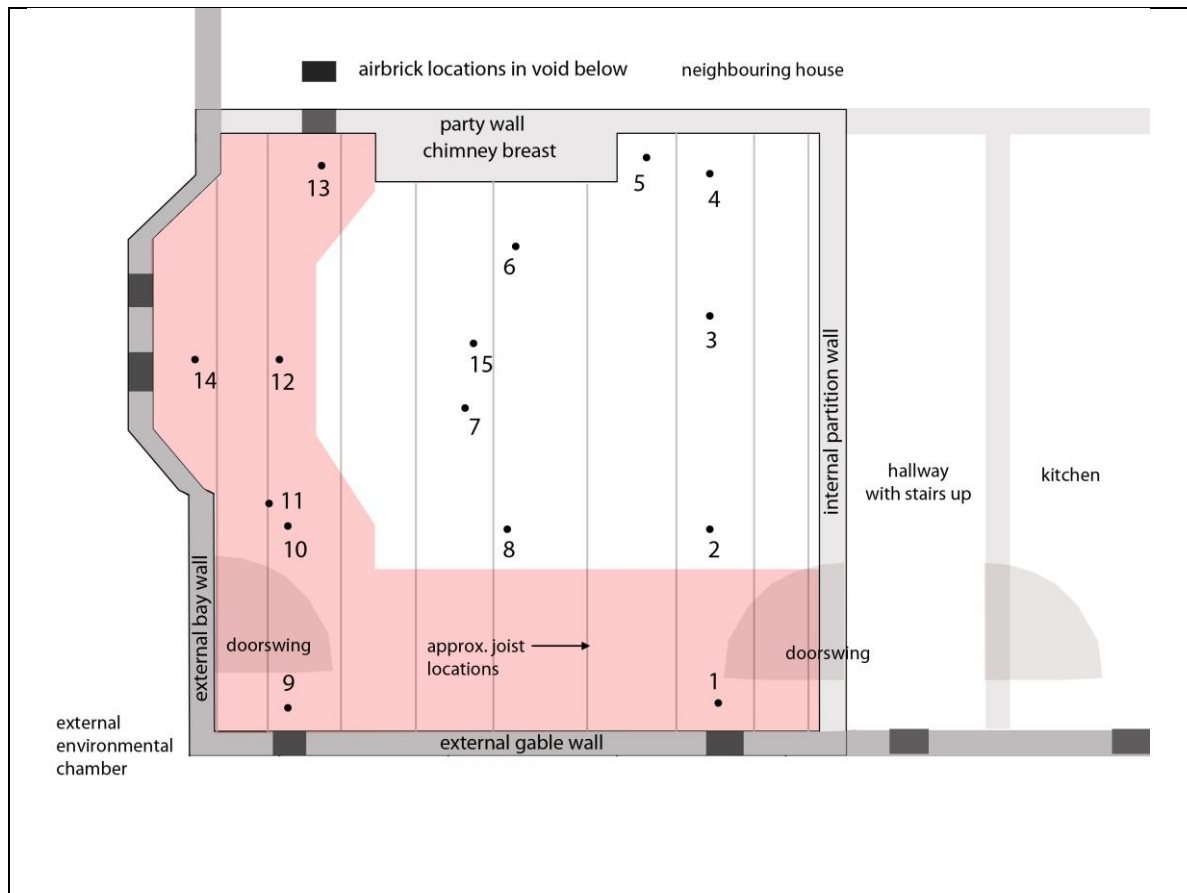
Fig. 1. Salford EH living room plan and in-situ point measurement locations; note that location 11 was taken on a joist; the shaded area signifies a 1 metre perimeter zone.
