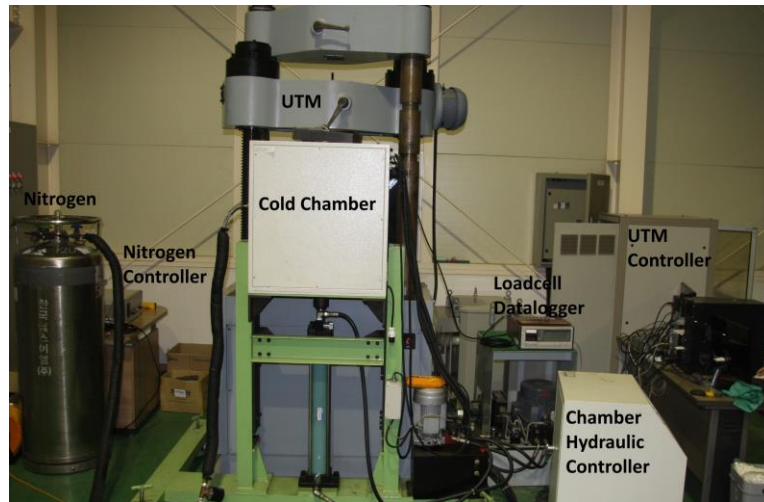
Figure 5. Test set-up for ice in compression at the Korea Ship and Offshore Research Institute at Pusan National University.
