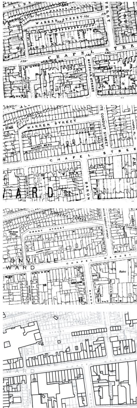
Figure 5. Chapel Street, Islington, London – historical building footprints showing terraced house transformations, from top to down: 1875, 1910, 1965, 2013. Historical and background maps: © 2013 Crown Copyright. An Ordnance Survey/EDINA supplied service.
