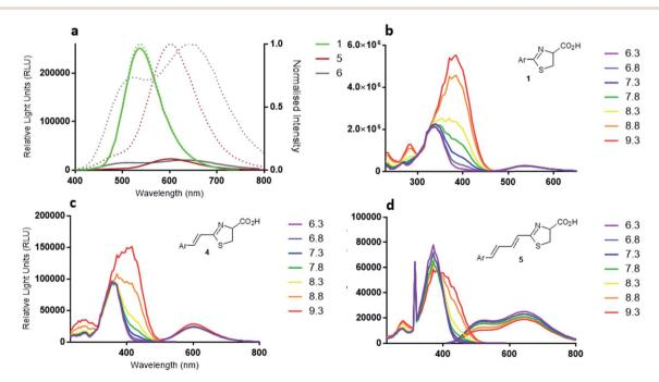
Fig. 3 (a) Fluorescence emission spectra of p-luciferin (1) (green line), infra-luciferin (4) (red line) and 5 (black line). Dotted lines are normalized spectra, (b) pH dependence of fluorescence spectra of p-luciferin (1) (330 nm excitation), (c) infra-luciferin (4) (352 nm excitation), and (d) 5 (369 nm excitation) measured in 5 nm increments.
