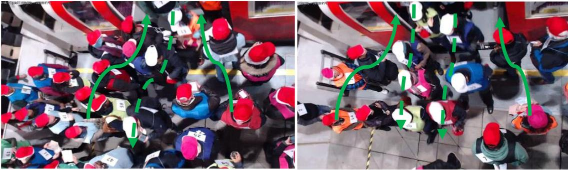
Figure 4. Formation of lanes when  $R = 4$  (left) and  $R = 0.25$  (right) at PAMELA
