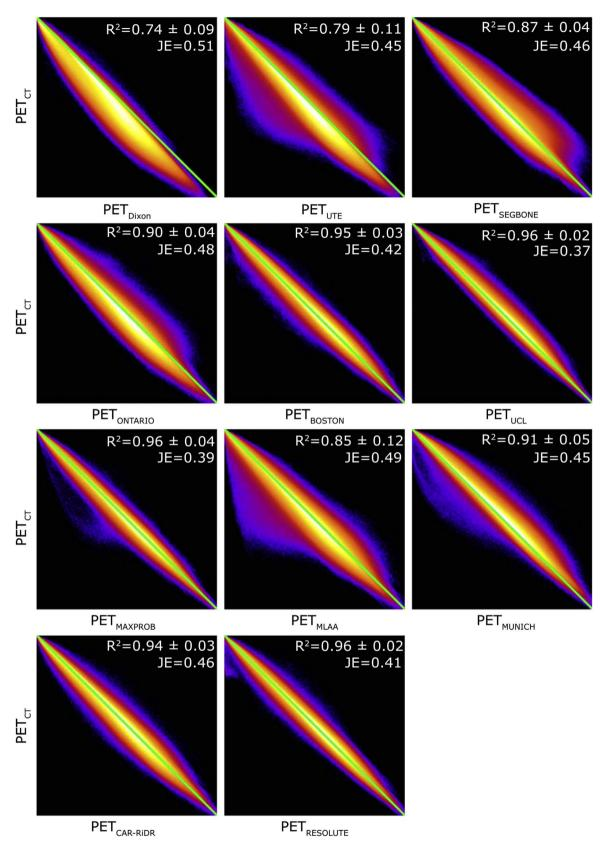
Fig. 4. Summed joint histograms of PET activity within the brain mask for FDG (n=192, excluding patients with fat/water tissue inversion) for  $PET_{CT}$  versus each of the methods. The R<sup>2</sup> scores are average ± SD of the individual patients. The joint entropy (JE) is calculated for all patients.
