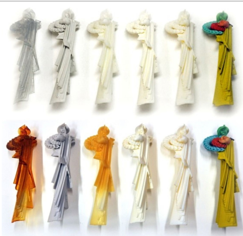
Fig. 1 Images of the RP artwork “Out of the Cauldron” designed by Tom Lomax produced with the most common RP Technologies: (1) stereolithography (SLA ® ) (2) polyjet (3) 3D printing (3DP) (4) selective laser sintering (SLS). Before ( above ) and after ( below ) photodegradation
