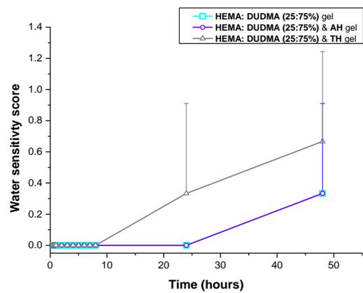
**Fig. 3.22** Water sensitivity score of UV-cured films produced from DUDMA & HEMA gels ( $\pm$  drug) with a DUDMA:HEMA ratio of 75:25% v/v. Means and standard deviations are shown, n=3.
