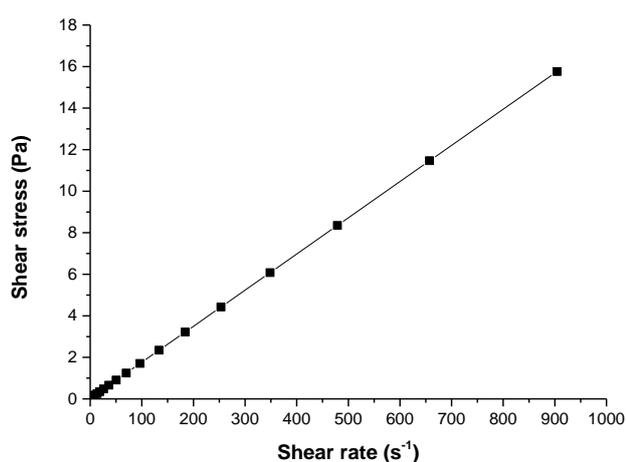
Fig. 2.2 Typical rheogram of UV-curable gel formulation
