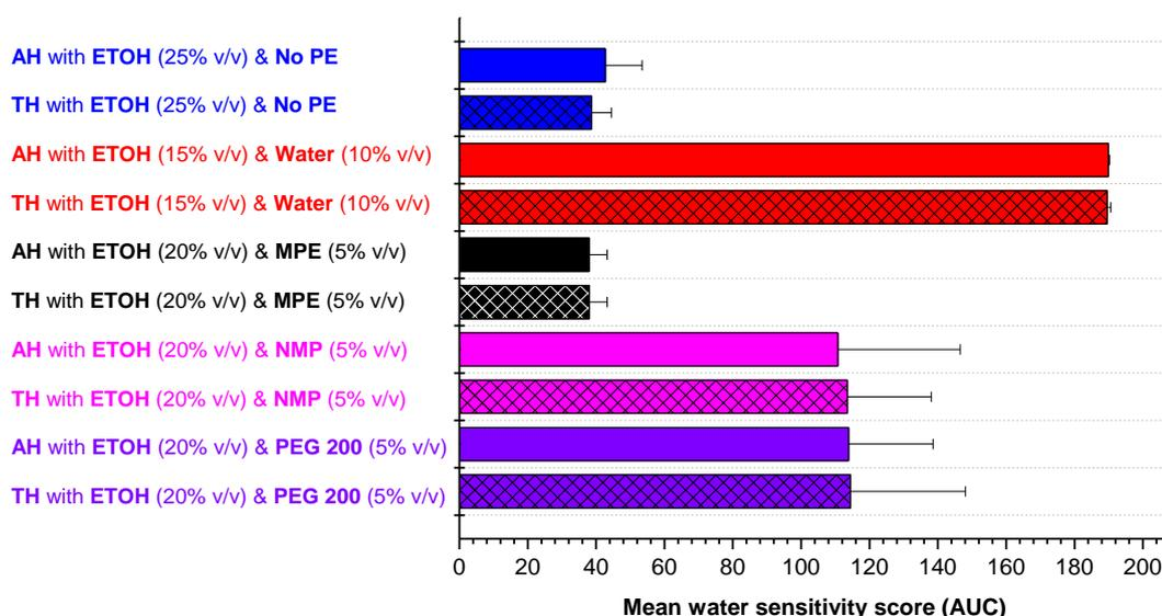
**Fig. 5.5** Area under the curve values calculated from the curves in Fig. 5.3 & Fig. 5.4 for the UV-cured films produced from the drug-loaded DUDMA & HEMA gels containing ethanol (ETOH) and different penetration enhancers (PE). Means and standard deviations are shown, n=3. AUC was determined using OriginPro 9.0.
