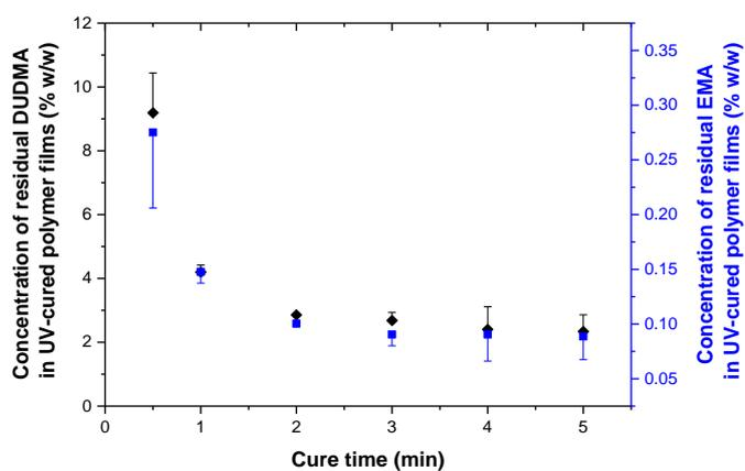
**Fig. 2.16** Effect of UVA cure-time on concentration of residual monomers in the cured polymer films. Means and standard deviations are shown, n=3.
