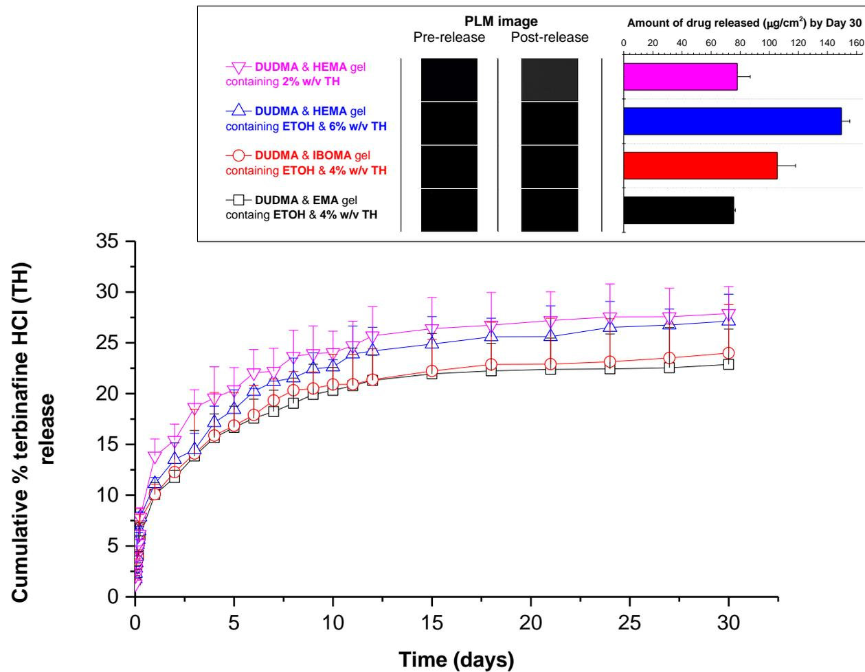
**Fig. 4.5** Cumulative % drug release from the terbinafine HCl loaded UV-cured films, their corresponding polarised light microscopy images (pre- and post-release) and the amount of drug released by day 30. Means and standard deviations are shown, n=3. Abbreviations: TH, terbinafine HCl; ETOH, ethanol.
