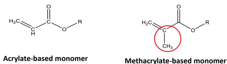
**Fig. 2.3** Chemical structure of acrylate and methacrylate-based monomers.
