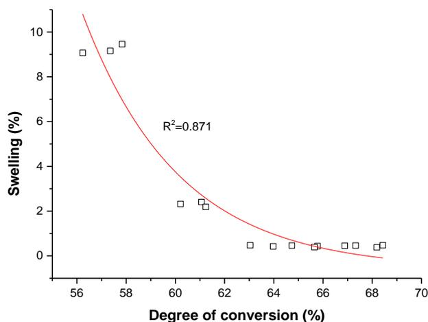
**Fig. 3.6** Influence of degree of conversion (%) from monomer gel to polymer film on the resulting film's swelling ability, and hence cross-linking extent.
