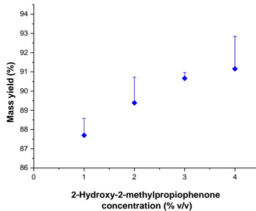
**Fig. 2.4** Effect of photoinitiator concentration on mass yield from monomer to cured polymer film. Means and standard deviations are shown,  $n=3$ . The Kruskal Wallis test with post hoc analysis performed with Nemenyi's test showed a significant increase in mass yield ( $p<0.05$ ) between a 1% and 4% photoinitiator concentration. All other differences were insignificant ( $p>0.05$ ).
