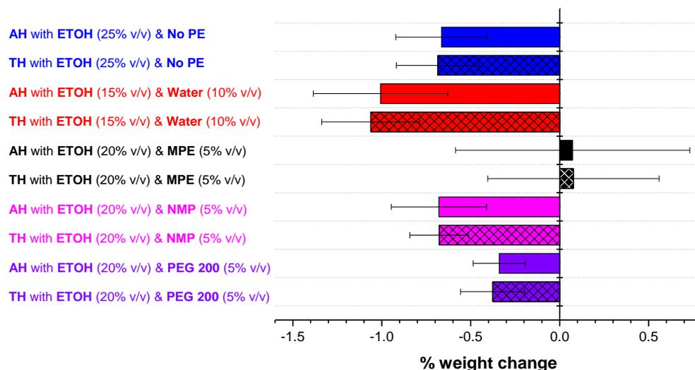
**Fig. 5.8** Weight change (%) for UV-cured films produced from drug-loaded DUDMA & HEMA gels containing ethanol (ETOH) and different penetration enhancers (PE) following drug-release studies. Means and standard deviations are shown, n=3. Abbreviations: AH, amorolfine HCl; TH, terbinafine HCl.
