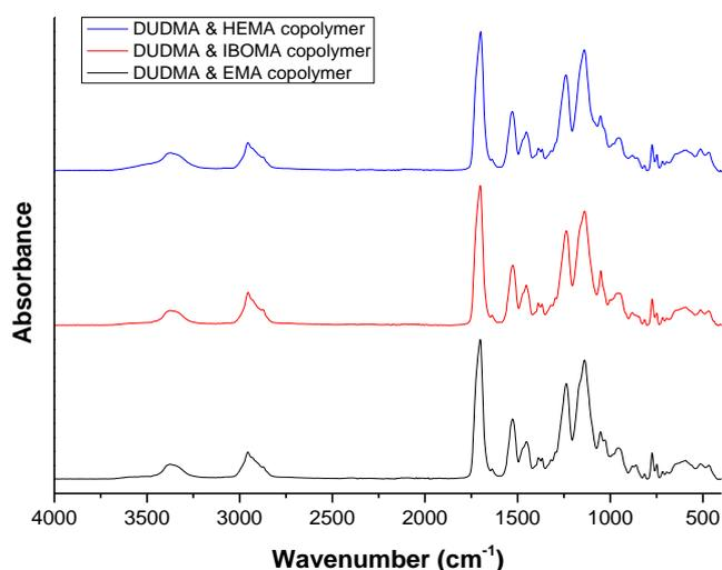
**Fig. 3.11** FT-IR spectra of DUDMA & EMA, IBOMA or HEMA copolymer films (drug-free and solvent-free with a DUDMA: diluent monomer ratio of 85:15% v/v).
