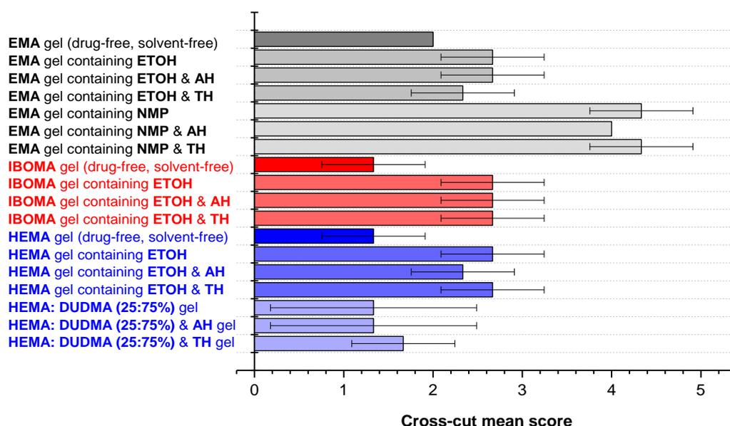
**Fig. 3.17** Cross-cut scores for films produced from gels containing DUDMA & EMA, IBOMA or HEMA ( $\pm$  solvent and  $\pm$  drug). Means and standard deviations are shown,  $n=5$ . High cross-cut scores mean lower adhesivity. Abbreviations: AH, amorolfine HCl; TH, terbinafine HCl; ETOH, ethanol.
