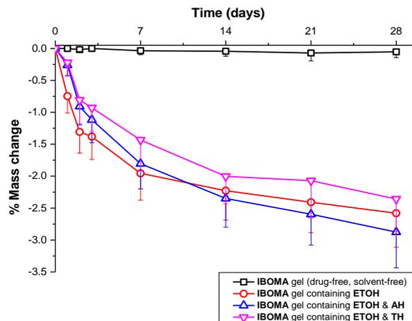
**Fig. 3.26** % Mass change of UV-cured films produced from DUDMA & IBOMA gels ( $\pm$  solvent and  $\pm$  drug). Means and standard deviations are shown, n=3.
