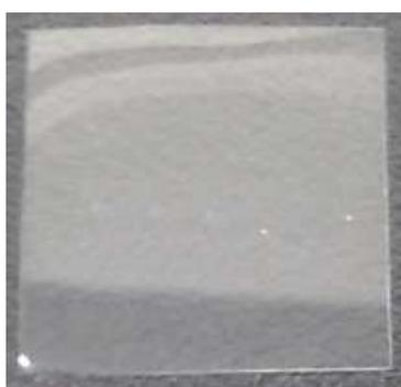
**Fig. 3.1** Photographic image of UV-cured film produced from a DUDMA & EMA containing gel formulation (drug-free and solvent-free).
