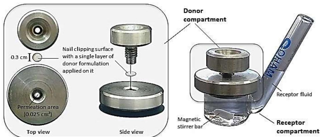
**Fig. 4.2** Modified Franz diffusion cell used for permeation studies. The donor compartment was made from steel and the receptor compartment from glass.
