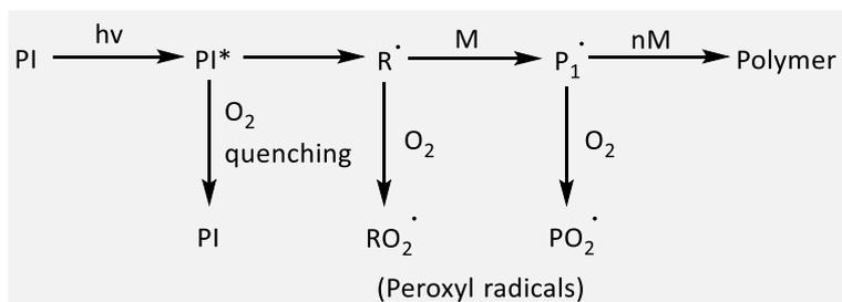
**Scheme 1** Oxygen inhibition in a radical-type photoinitiated polymerisation reaction. Abbreviations: PI, photoinitiator; M, monomer. (Adapted from Studer et al., *Progress in Organic Coatings* 48, 2003).
