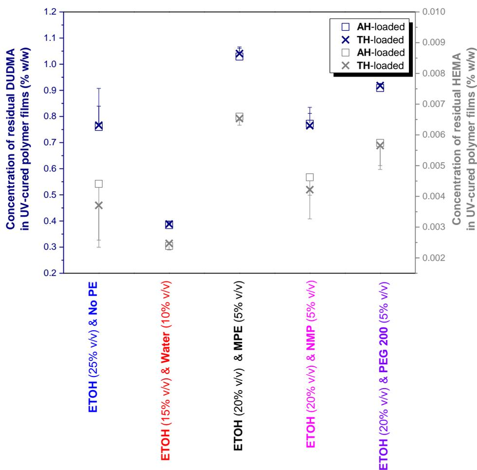
**Fig. 5.1** Influence of penetration enhancer incorporation on concentration of residual monomers in AH- or TH- loaded UV-cured DUDMA & HEMA copolymer films. Means and standard deviations are shown, n=3.
