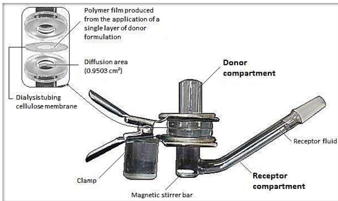
**Fig. 4.1** Franz diffusion cell set up for release studies. The cellulose membrane was only used to support the Curanail® film. UV-cured films did not need any support.
