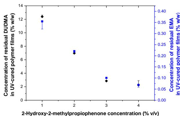
**Fig. 2.6** Effect of photoinitiator concentration on concentration of residual DUDMA and EMA monomers extracted from UV-cured polymer film. Mean levels of monomers in film and standard deviations are shown,  $n=3$ . There was no significant decrease in the amount of residual monomers extracted ( $p>0.05$ ) between a 3% and 4% photoinitiator concentration. All other differences were significant ( $p<0.05$ ).
