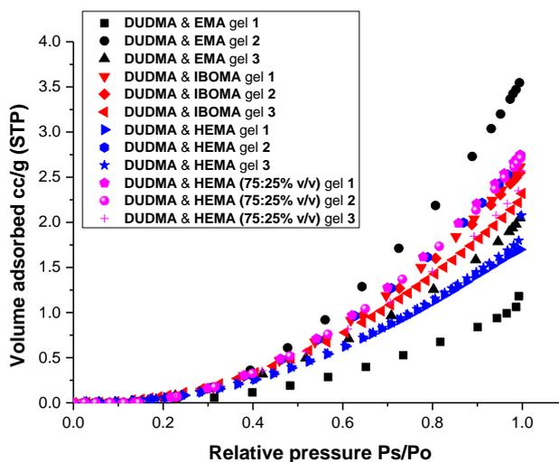
**Fig. 3.7** Relative pressure vs volume adsorbed for UV-cured films produced from DUDMA & EMA, IBOMA or HEMA containing gels (drug-free, solvent-free, with a DUDMA: diluent monomer ratio of 85:15 % v/v unless otherwise stated).
