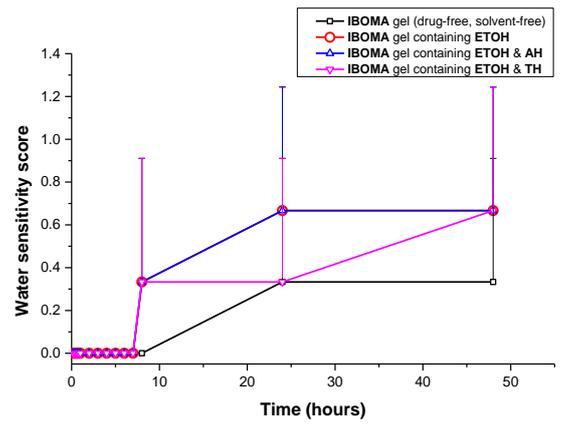
**Fig. 3.20** Water sensitivity score of UV-cured films produced from DUDMA & IBOMA gels ( $\pm$  solvent and  $\pm$  drug). Means and standard deviations are shown, n=3.
