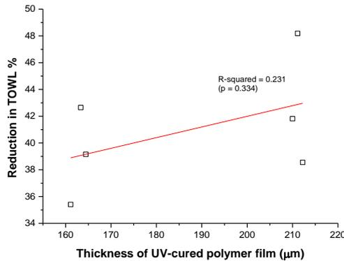
**Fig. 3.16** Influence of film thickness on film occlusivity. Greater reduction in TOWL % = greater occlusivity.
