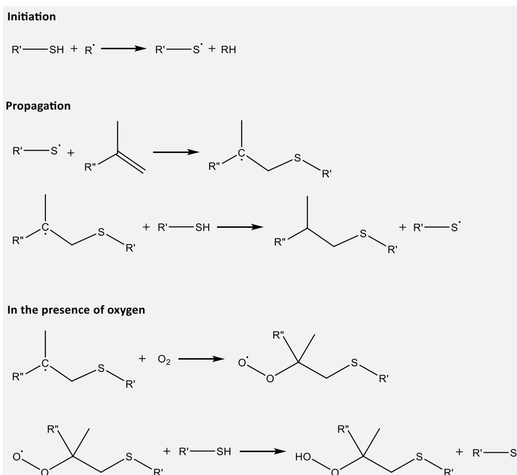
**Scheme 2** Thiols in a radical-type photoinitiated polymerisation reaction. (Adapted from Ligon et al., *Chemical Reviews*, 114, 1, 2014).
