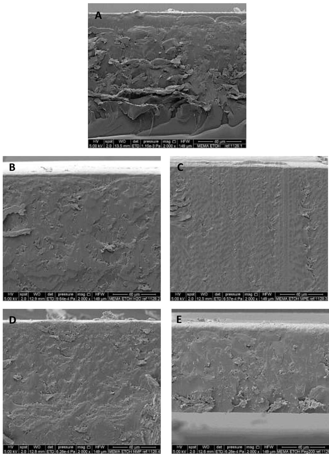
**Fig. 5.2** Scanning electron micrographs of the cross-sectional surfaces of UV-cured films produced from amorphine HCl-loaded DUDMA & HEMA gels containing ethanol and (A) no enhancer, (B) water, (C) MPE, (D) NMP and (E) PEG 200.
