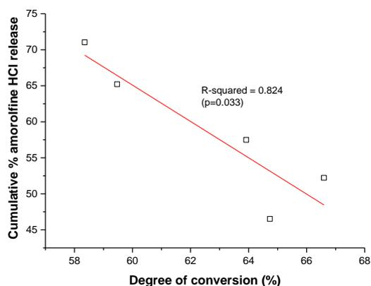
**Fig. 5.9** Influence of degree of conversion from monomer gel to polymer film on amorolfine HCl release from the polymer film.
