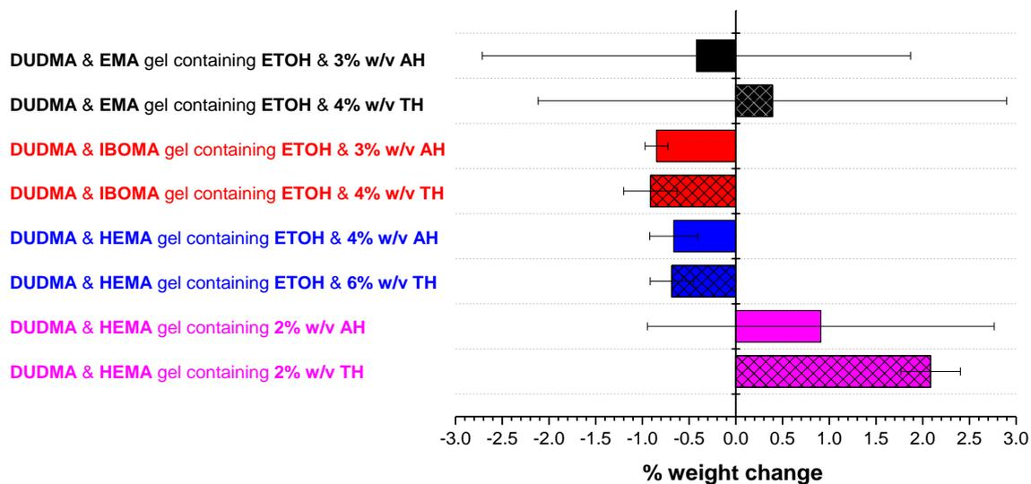
**Fig. 4.6** Weight change (%) for the drug-loaded UV-cured films produced from DUDMA & EMA, IBOMA or HEMA containing gels following drug-release studies. Means and standard deviations are shown, n=3. Abbreviations: AH, amorolfine HCl; TH, terbinafine HCl; ETOH, ethanol.
