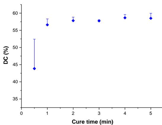
**Fig. 2.15** Effect of UVA cure-time on percentage DC from monomer to polymer. Means and standard deviations are shown, n=3.
