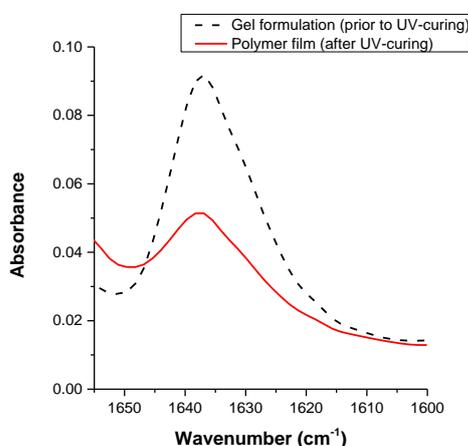
**Fig. 2.19** FT-IR spectra of the gel (containing DUDMA, EMA and photoinitiator) and of the resulting polymer film after UV-curing (but before removal of the oxygen inhibition layer).
