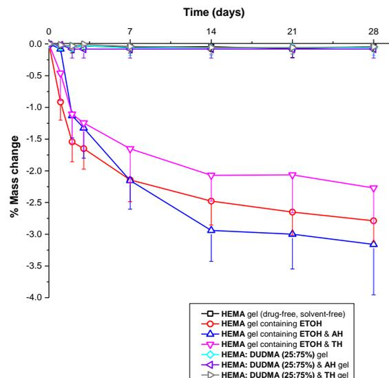
**Fig. 3.27** % Mass change of UV-cured films produced from DUDMA & HEMA gels ( $\pm$  solvent and  $\pm$  drug). Means and standard deviations are shown, n=3.
