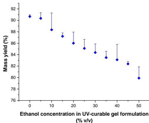
**Fig. 2.9** Percentage mass yield of films produced by UV-curable gel formulations containing between 0 and 50% v/v ethanol. Means and standard deviations are shown, n=3.
