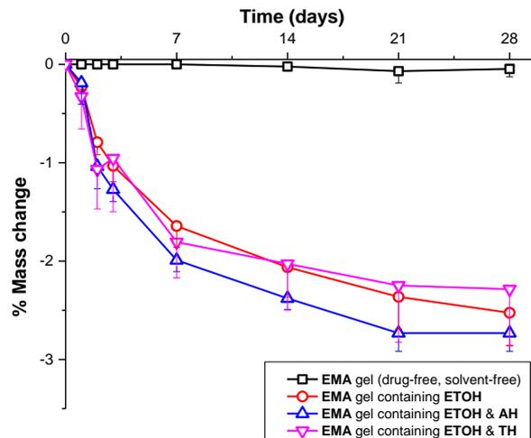
**Fig. 3.25** % Mass change of UV-cured films produced from DUDMA & EMA gels ( $\pm$  solvent and  $\pm$  drug). Means and standard deviations are shown, n=3.
