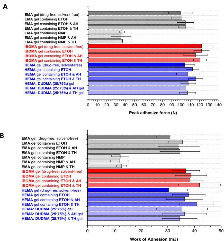
**Fig. 3.18** Peak adhesive force (A) and work of adhesion (B) readings obtained for the UV-cured films produced from gels containing DUDMA & EMA, IBOMA or HEMA ( $\pm$  solvent and  $\pm$  drug). Means and standard deviations are shown, n=3.
