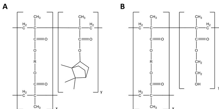
**Fig. 2.18** Basic chemical structure of A) DUDMA & IBOMA copolymer and B) DUDMA & HEMA copolymer.
