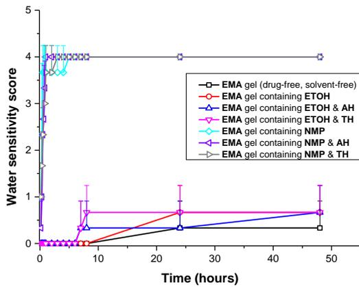
**Fig. 3.19** Water sensitivity score of UV-cured films produced from DUDMA & EMA gels ( $\pm$  solvent and  $\pm$  drug). Means and standard deviations are shown, n=3.
