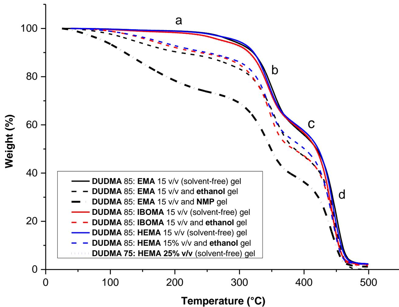
**Fig. 3.12** TGA profiles of films produced from drug-free UV-curable gel formulations containing EMA, IBOMA and HEMA represented by black, red and blue respectively.
