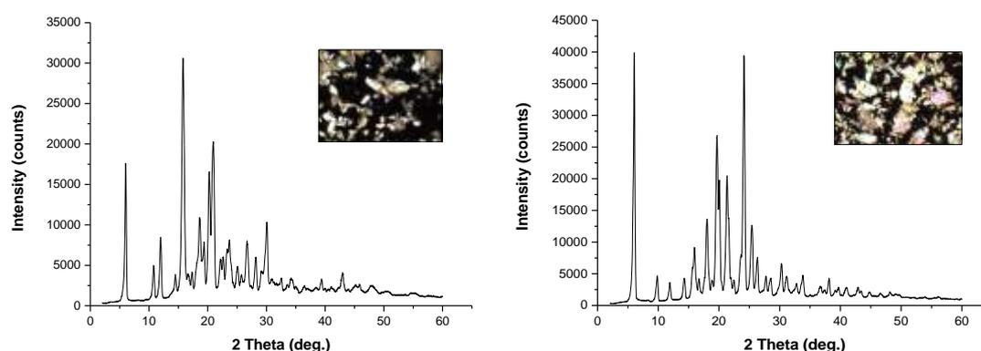
**Fig. 3.9** Polarised light micrograph & corresponding XRD pattern of amorolfine HCl (left) & terbinafine HCl (right).
