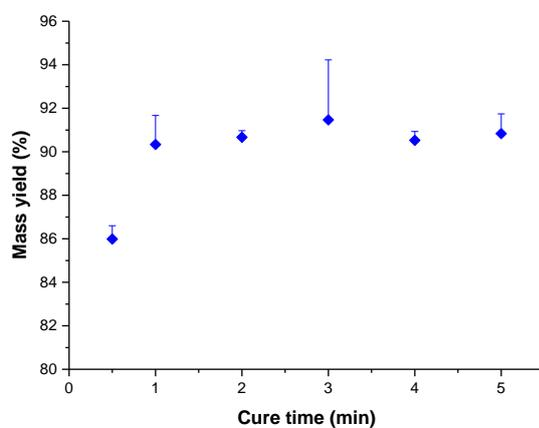
**Fig. 2.14** Effect of UVA cure-time on mass yield from monomer to cured polymer film. Means and standard deviations are shown, n=3.
