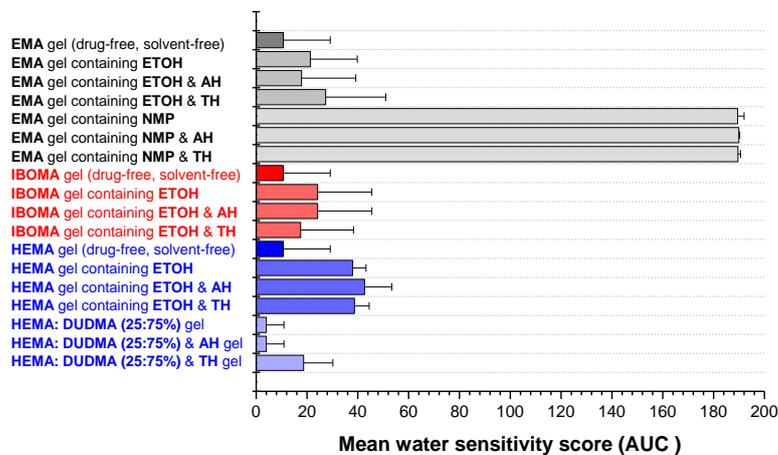
**Fig. 3.23** Area under the curve values calculated from the curves in Fig. 3.19 – Fig. 3.22 for the UV-cured films produced from DUDMA & EMA, IBOMA or HEMA containing gels ( $\pm$  solvent and  $\pm$  drug). Means and standard deviations are shown, n=3. AUC was determined using OriginPro 9.0.
