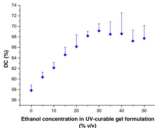
**Fig. 2.7** Percentage DC from monomer to polymer for formulations containing between 0 and 50% v/v ethanol. Means and standard deviations are shown, n=3.
