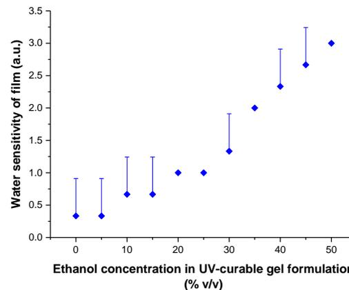
**Fig. 2.10** Water sensitivity (at 48 hour incubation) of films produced by UV-curable gel formulations containing between 0 and 50% v/v ethanol. Means and standard deviations are shown, n=3.
