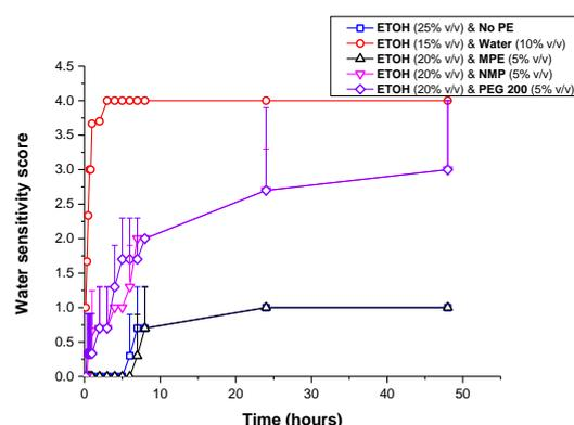
**Fig. 5.4** Water sensitivity scores for terbinafine HCl-loaded UV-cured films produced from DUDMA & HEMA gels containing ethanol (ETOH) and different penetration enhancers (PE). Means and standard deviations are shown, n=3.
