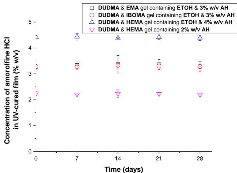
**Fig. 3.28** Stability of amorphine HCl in UV-curable films over time. Means  $\pm$  standard deviations are shown, n=3. Abbreviations: AH, amorphine HCl; ETOH, ethanol.
