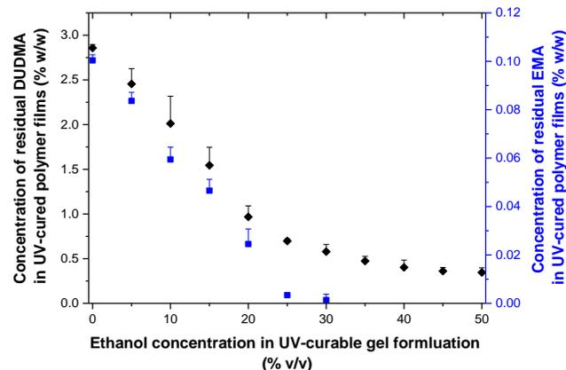
**Fig. 2.8** Concentration of residual monomers in the UV-cured polymer films produced from formulations containing between 0 and 50% v/v ethanol. Means and standard deviations are shown, n=3.
