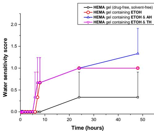
**Fig. 3.21** Water sensitivity score of UV-cured films produced from DUDMA & HEMA gels ( $\pm$  solvent and  $\pm$  drug). Means and standard deviations are shown, n=3.
