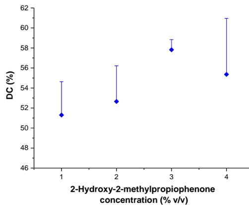
**Fig. 2.5** Effect of photoinitiator concentration on percentage DC from monomer to polymer. Means and standard deviations are shown,  $n=3$ . The Kruskal Wallis test with post hoc analysis performed with Nemenyi's test showed no significant increase in DC % ( $p>0.05$ ) as the concentration of the photoinitiator increased.
