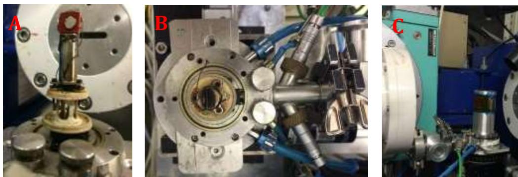
Figure 6.1: Left to right A) In situ high temperature cell, B) View from the top of the in situ cell, C) The cap of the in situ cell that allowed for a He flow throughout the course of the reactions.
