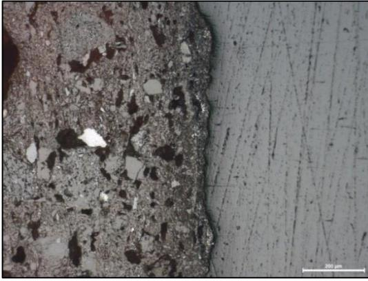
Figure 7.30 Photomicrograph of sample 108-6857 cross section showing the purple-coloured layer on the surface of the ceramic under plane-polarized light.
