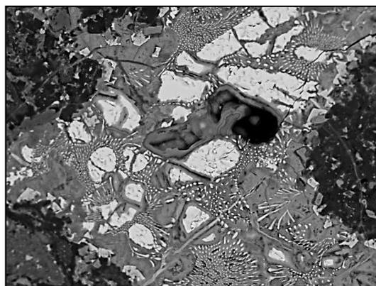
**Figure 7.71** SEM image of sample 630-3865 showing the various phases of partially corroded HSS. The bright grey angular phases are pyrrhotite and covellite while the small fine finger-like structures at the grain boundaries are magnetite.
