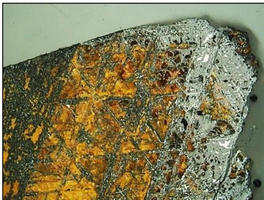
Figure 7.44 Photomicrograph of sample 257-3130. The bright whitish phases are the remaining chalcopyrite crystals surrounded by corrosion. Entirely missing are the pyrite crystals which have largely corroded to iron oxides, leaving behind only the crystalline structure.
