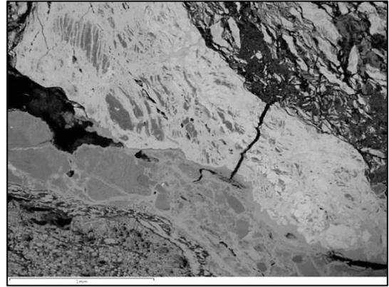
Figure 7.88 SEM image of sample 97-3588's mixed matrix. In the bottom right is a large fragment of silicified charcoal while in the top right is a large fragment of copper-bearing goethite. Between them is fayalitic slag.
