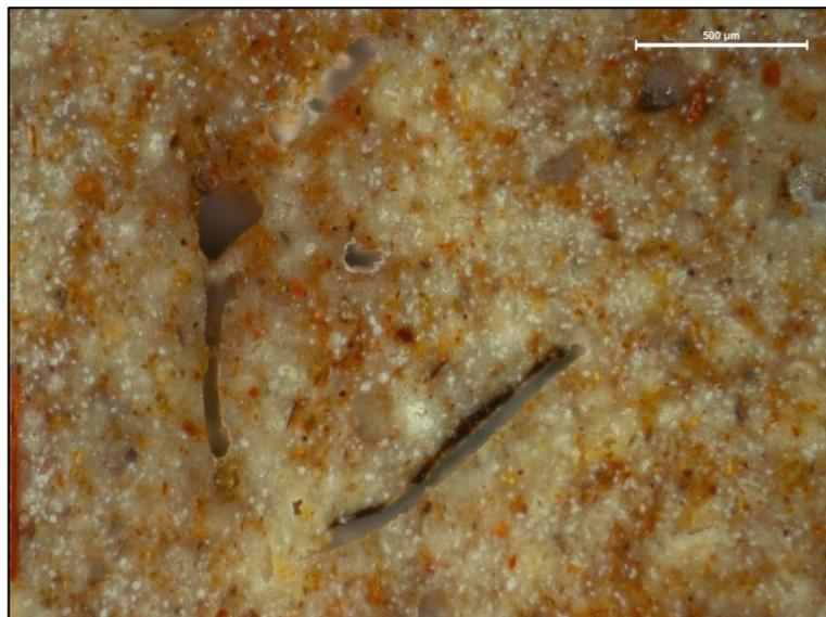
**Figure 7.111** Photomicrograph of furnace wall sample FG-030670 with typical organic temper voids. Although the matrix here is relatively fine grained and thus poor in mineral inclusions, the rest of the sample does contain significant quantity of them.
