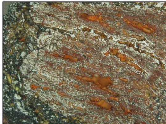
Figure 7.43 Photomicrograph of sample 753-5028 with both magnetite and iron hydroxides within the porosities.
