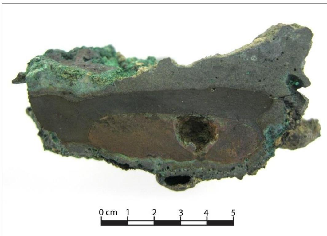
**Figure 7.150** Photograph of cross section of sample FG-012260B. The layering of metallic copper, matte, and slag can be clearly seen as it must have been in the larger slag cakes from Arisman.
