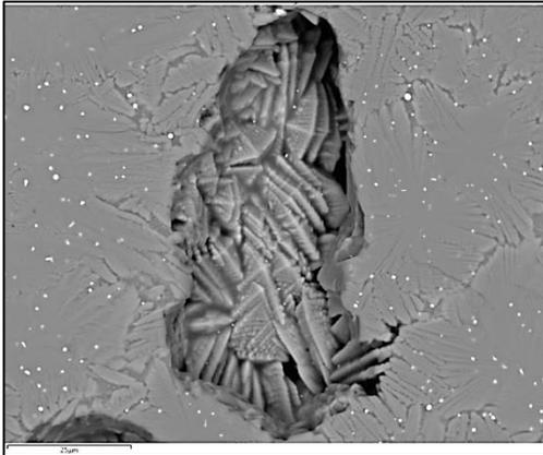
Figure 7.165 SEM image of sample FG-030974D's microcrystalline matrix. The dendrites are near hedenbergite in composition. The large porosity in the centre shows the three-dimensional structure of the dendrites. The small bright prills are copper metal and copper sulphide.
