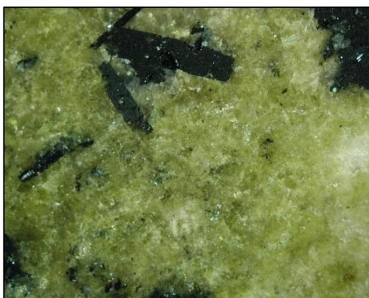
Figure 7.131 Photomicrograph of Sample FG-011992 in cross-polarized reflected light. The dark angular crystals are magnetite while the matrix is mainly composed of greenish anorthite while the white blebs are calcium carbonate. Frame is 2.4mm wide.
