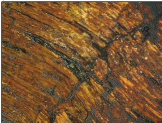
Figure 7.42 Photomicrograph of sample 585-4328A showing a network of elongated iron hydroxide crystals.
