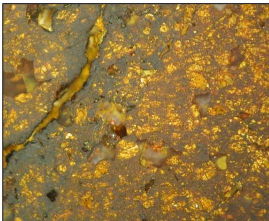
Figure 7.133 Photomicrograph of sample FG-030125 under cross-polarized reflected light. The grey phases are iron oxide while the yellow phases are iron sulphide. The sulphide phases appear under the microscope mainly in the porosities, still visible through the clear resin. Frame is 1.2mm wide.
