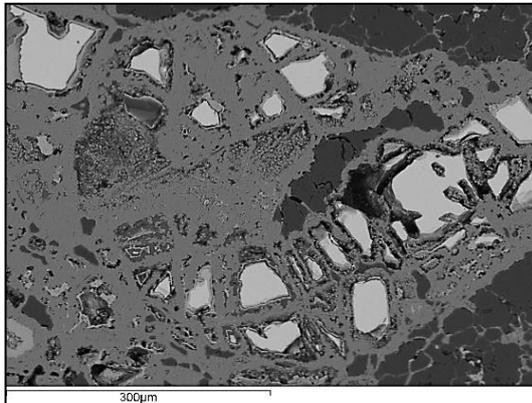
Figure 7.40 SEM image of sample 799-5409. The bright grey angular crystals are chalcopyrite surrounded by light grey corrosion in a dark grey quartz matrix.
