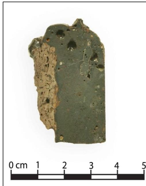
**Figure 7.136** Cross section of speiss slag fragment with attached furnace remains. This specimen is the only one of the speiss slags to show minimal porosity. Sample FG-040919B.
