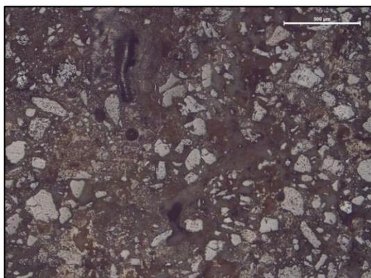
**Figure 7.115** Plane polarized photomicrograph of sample FG-012232 showing typical technical ceramic microstructure.
