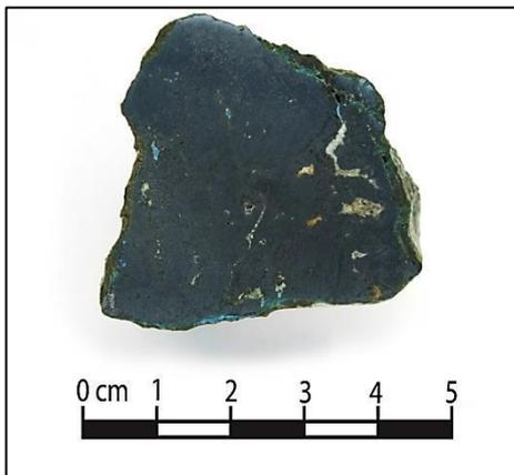
Figure 7.168 Photograph of sample FG-030689's cross section. Note the large inclusions visible throughout.
