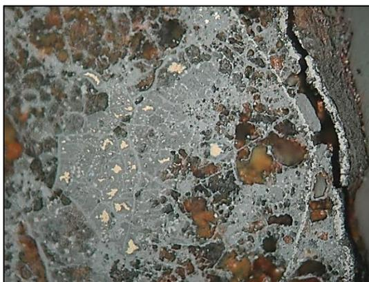
Figure 7.50 Photomicrograph of sample 619-3497 showing the original pyrite and chalcopyrite mineral microstructure. The pinkish colours are chalcopyrite while the grey is iron silicate and the light grey is magnetite. Orange iron hydroxides can be seen throughout where the mineral has weathered post-depositionally.
