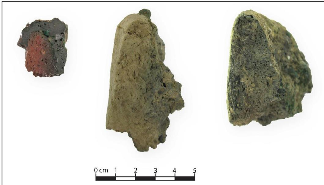
**Figure 7.112** Three furnace fragment samples with rims. All show extensive heat damage applied mainly to the inside but extending deep into the fabric. Note two distinct layers of slag on the leftmost example, with the top layer extending over the edge and most likely deposited after the ceramic had been broken and discarded.
