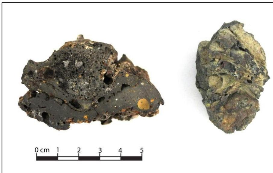
Figure 7.135 Photographs of two samples showing the typical features associated with speiss slag. Note the orange and yellow corrosion staining on the surface and in the pores. Also note the layered and flowing surface features typical of tapped slag. The sample on the left is FG-010506 while that on the right is FG-030123B.
