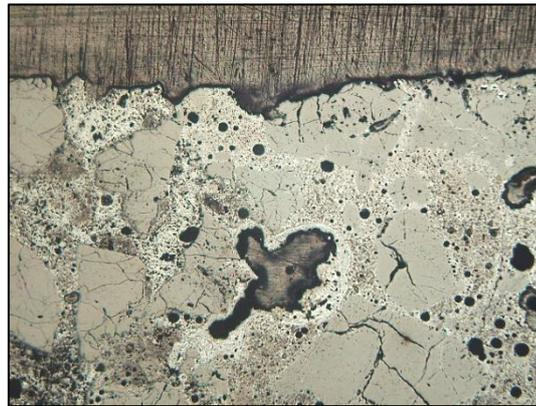
**Figure 7.73** SEM image of sample 222-326A. The large angular grey cracked crystals are quartz while the surrounding microcrystalline matrix is mainly composed of magnetite and olivines.
