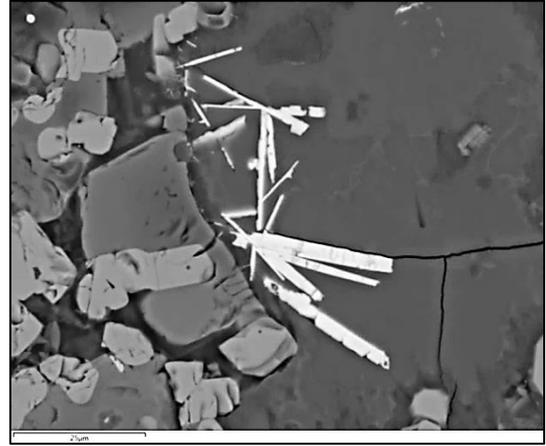
Figure 7.67 SEM image of sample 890-5774 showing elongated lath-like barite/celestine crystals growing within a cavity. The surrounding matrix is composed of dark grey fayalite and light grey magnetite.
