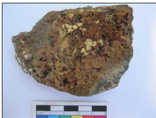
Figure 7.24 Pottery sample 200-6526 with 1cm thick crust of iron hydroxide corrosion on the surface.
