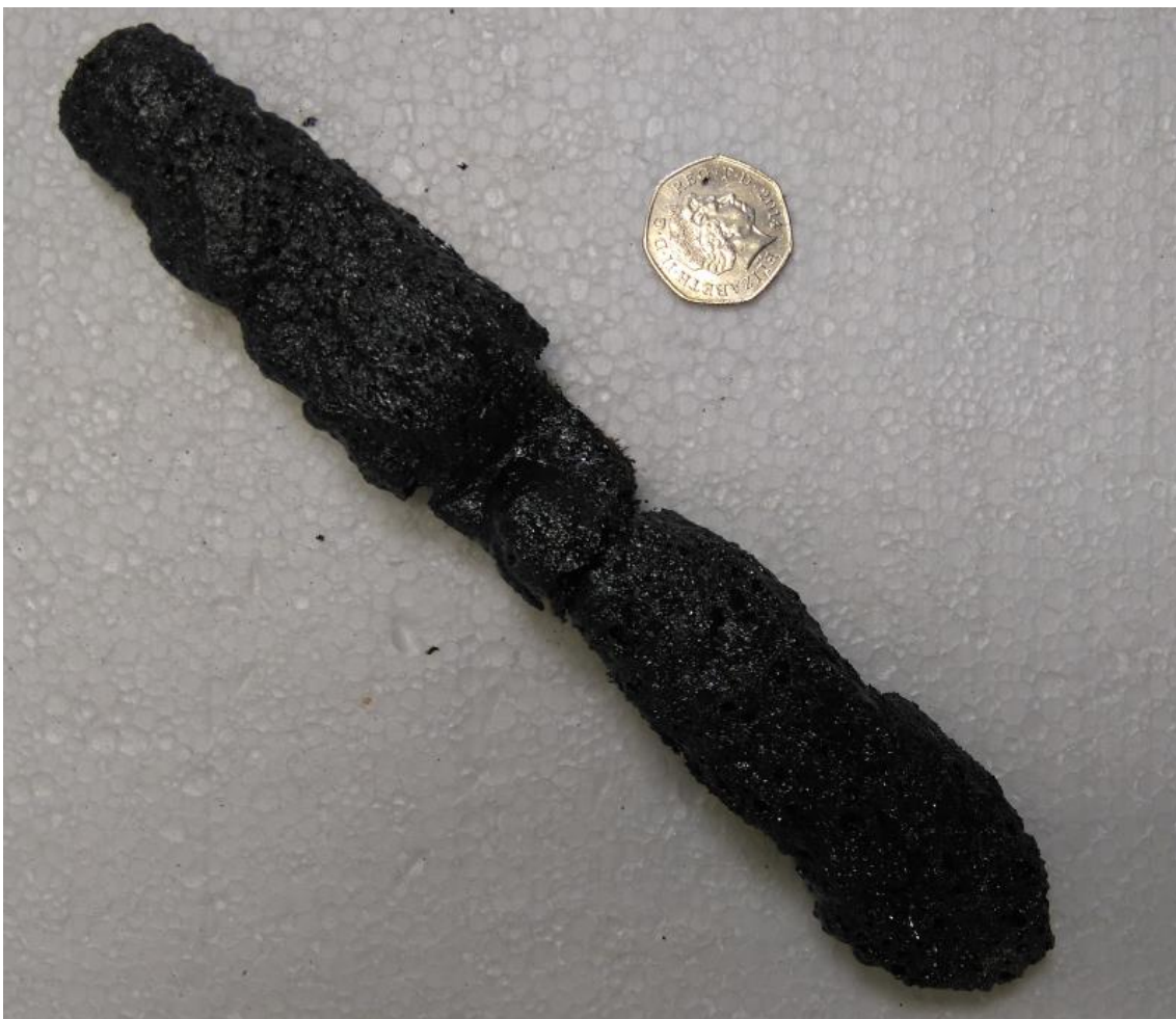
Figure S6. Photograph of a large sulfur-carbon monolith synthesised from annealing 20 g of ground 50 wt. % DIB polymer at 750 °C for 1 hour under N 2 . For scale, a UK 50 pence piece is added.
