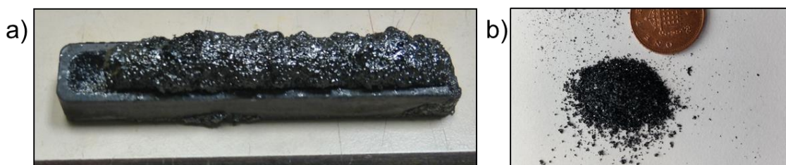
Figure S7. a) Photograph of a sulfur-carbon monolith synthesised from annealing 4 g of 50 wt. % Limonene polymer at 750 °C for 1 hour under N 2 . b) powdered form of the carbonised S-limonene polymer after breaking it up for sorption analysis.
