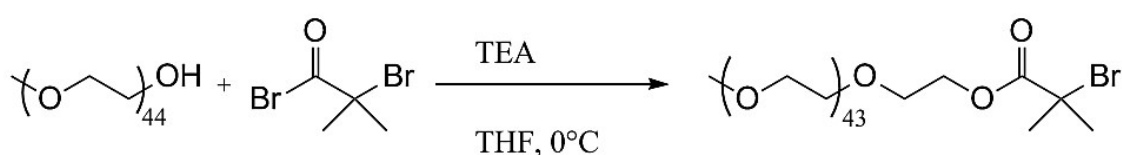
Figure S1. Schematic representation of the esterification reaction of PEG using BIBB.
