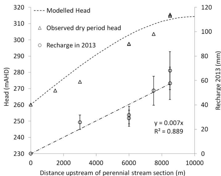
**Figure 10.** Variation of estimated recharge with distance upstream and comparison of observed dry period heads (i.e., during a straight line recession period) with heads predicted using equation (4).
