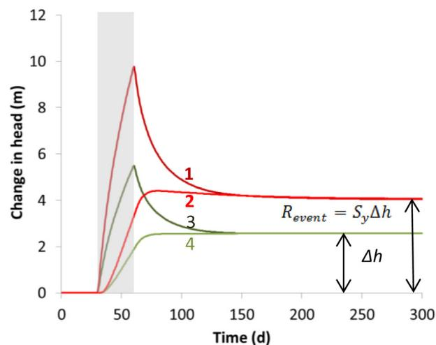
**Figure 5.** Groundwater hydrographs for the cases shown in Figure 2 with the long-term recession removed to reveal the effects solely due to recharge from the stream. Grey shading indicates the period of steady flux input at the stream boundary.
