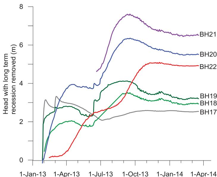
**Figure 8.** Groundwater hydrographs with background recessions “removed.” The final head value represents the increase due to recharge from ephemeral streamflow since January 2013. Where continuous data were not available from data loggers (i.e., BH22, BH19, and BH21), the residual heads were calculated using dip-tape measurements taken just prior to the streamflow event in late January 2013.
