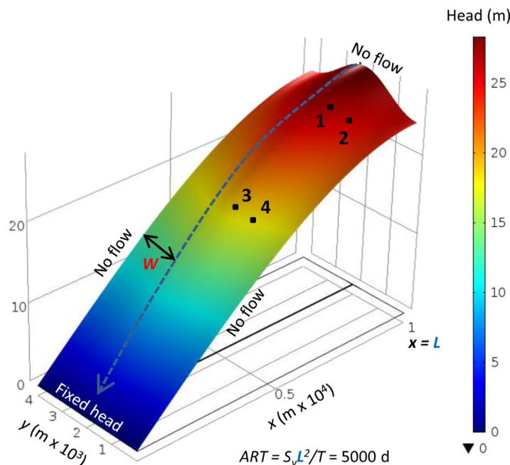
**Figure 1.** Model of an idealized aquifer receiving indirect recharge from an ephemeral stream. The parameters used were as follows:  $T = 200 \text{ m}^2/\text{d}$ ,  $S_y = 0.01$ . Dashed blue arrow represents the stream recharge boundary. Heads are relative to the fixed head boundary at  $x = 0$  and represent the water table during a streamflow/recharge event. Numbers 1–4 are locations that represent the computed groundwater hydrographs in Figure 2.
