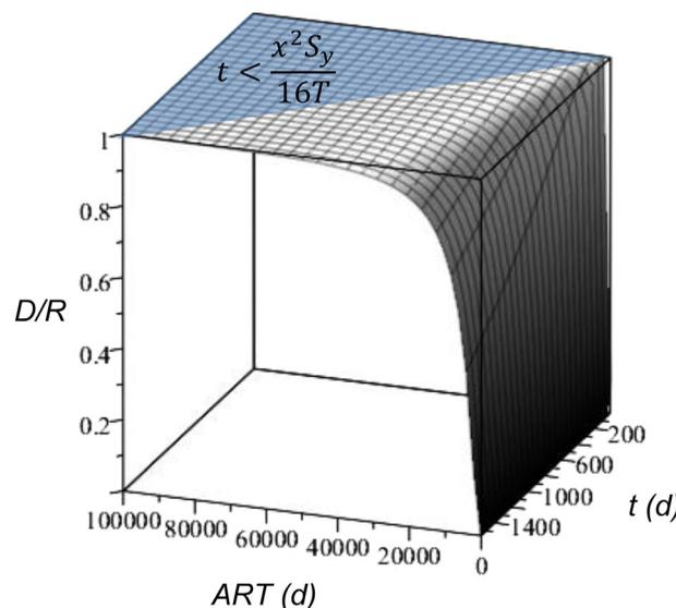
**Figure 3.** Rates of groundwater flux recession ( $D$ ) after recharge ceases normalized to the recharge rate ( $R$ ) used to determine the initial conditions, for variations in aquifer response time ( $ART = S_yL^2/T$ ) and time, for a groundwater monitoring point positioned at  $x = 0.5L$ . Shaded zone is for  $t < t_{lin}$  as defined by Cuthbert [2014].
