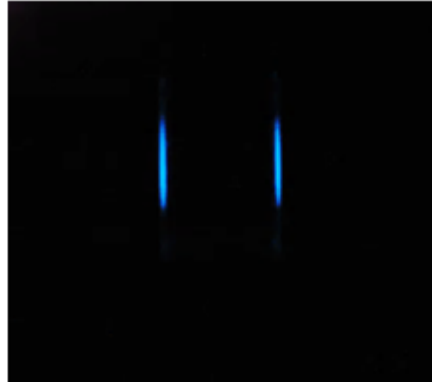
Figure 20: Interface issue – the PMMA container wall was found to be scintillating when left empty.
