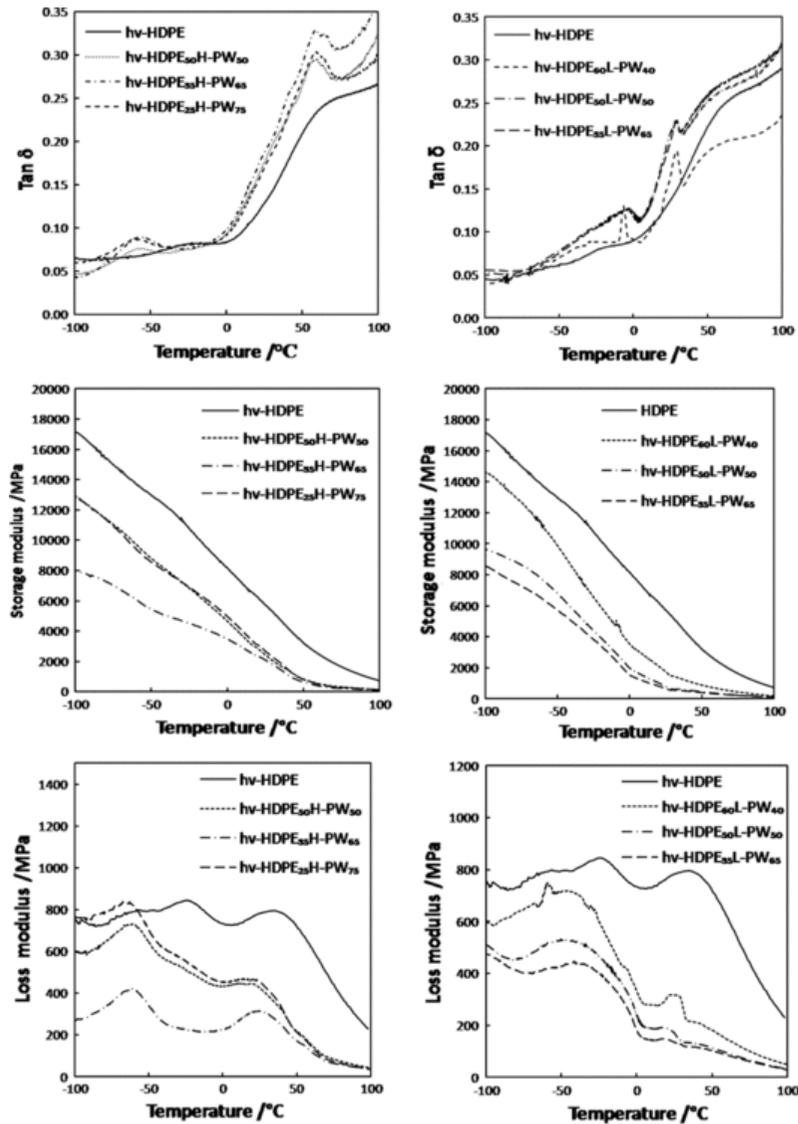
**Fig. 6** DMTA results of (a)  $\tan \delta$  of hv-HDPE and hv-HDPE/H-PW blends; (b)  $\tan \delta$  of hv-HDPE and hv-HDPE/L-PW blends; (c) storage modulus ( $E'$ ) for hv-HDPE and hv-HDPE/H-PW blends; (d)  $E'$  for hv-HDPE and hv-HDPE/L-PW blends; (e) loss modulus ( $E''$ ) of hv-HDPE and hv-HDPE/H-PW blends; (f)  $E''$  of hv-HDPE and hv-HDPE/L-PW blends, as a function of temperature.
