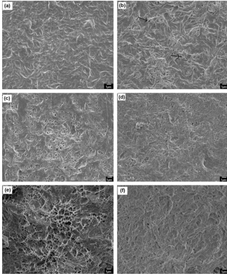
**Fig. 1** SEM images of (a) surface of hv-HDPE<sub>35</sub>H-PW<sub>65</sub>; (b) surface of hv-HDPE<sub>35</sub>H-LW<sub>65</sub>; (c) surface of hv-HDPE<sub>35</sub>H-PW<sub>65</sub> after xylene treatment; (d) surface of hv-HDPE<sub>35</sub>H-PW<sub>65</sub> after xylene treatment; (e) fractured surface of hv-HDPE<sub>35</sub>H-PW<sub>65</sub> and (f) fractured surface of hv-HDPE<sub>35</sub>H-PW<sub>65</sub>.
