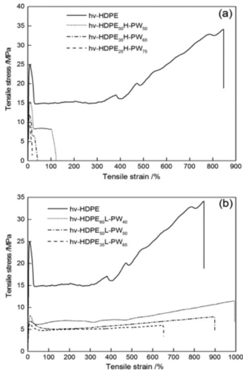
**Fig. 8** Stress–strain curves of (a) hv-HDPE and hv-HDPE/H-PW blends and (b) hv-HDPE and hv-HDPE/L-PW blends.
