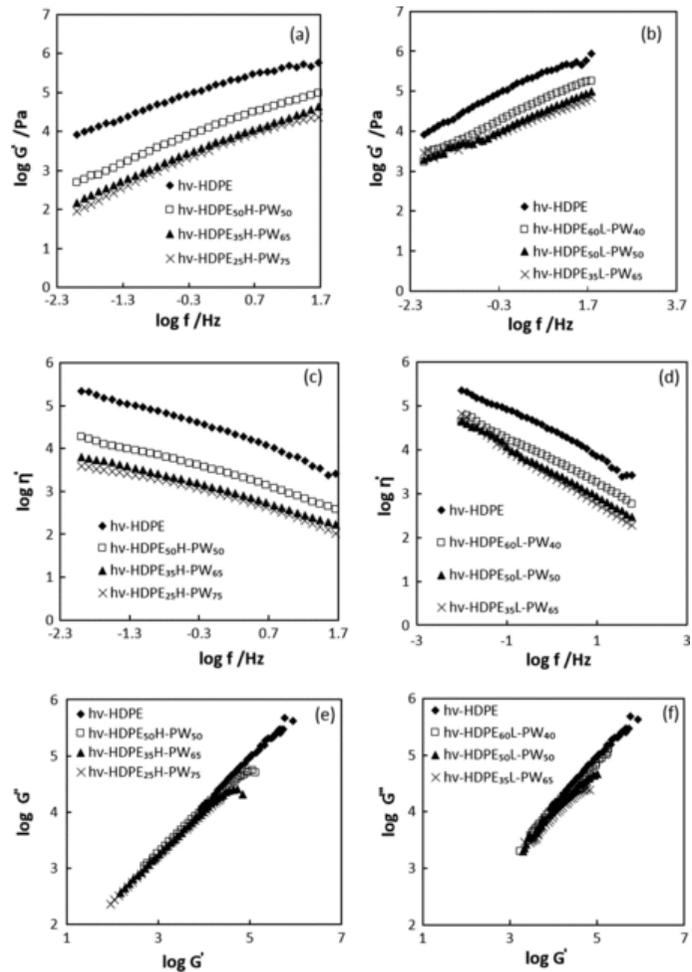
**Fig. 12** Oscillatory rheology: plots of  $\log G'$  versus  $\log f$  for (a) hv-HDPE and hv-HDPE/H-PW blends and (b) hv-HDPE and hv-HDPE/L-PW blends; plots of  $\log \eta'$  versus  $\log f$  plot of (c) hv-HDPE and hv-HDPE/H-PW blends and (d) hv-HDPE and hv-HDPE/L-PW blends; plots of  $\log G'$  versus  $\log G''$  (Cole–Cole plots) for (e) hv-HDPE and hv-HDPE/H-PW blends and (f) hv-HDPE and hv-HDPE/L-PW blends, at 160 °C.
