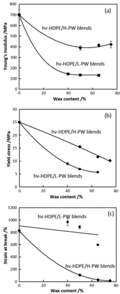
Fig. 7 Tensile testing results of variation in (a) Young's modulus, (b) yield stress and (c) strain at break of hv-HDPE, hv-HDPE/H-PW and hv-HDPE/L-PW blends, as a function of wax content.
