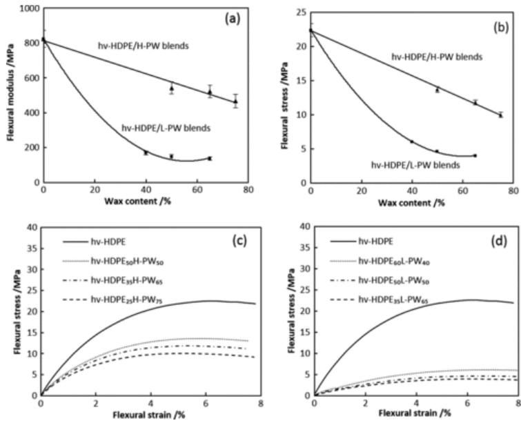
Fig. 9 Flexural testing results of variation in (a) flexural modulus and (b) flexural stress of hv-HDPE, hv-HDPE/H-PW and hv-HDPE/L-PW blends, as a function of wax content; stress–strain curves for (c) hv-HDPE and hv-HDPE/H-PW blends and (d) hv-HDPE and hv-HDPE/L-PW blends.
