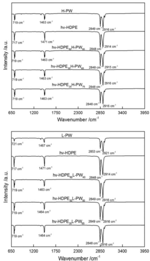
**Fig. 2** FTIR spectra of (a) H-PW, hv-HDPE and hv-HDPE/H-PW blends, and (b) L-PW, hv-HDPE and hv-HDPE/L-PW blends.
