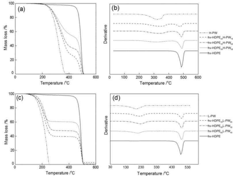
**Fig. 5** TGA curves for (a) H-PW, hv-HDPE and hv-HDPE/H-PW blends; DTG curves for (b) H-PW, hv-HDPE and hv-HDPE/H-PW blends; TGA curves for (c) L-PW, hv-HDPE and hv-HDPE/L-PW blends and DTG curves for (d) L-PW, hv-HDPE and hv-HDPE/L-PW blends.
