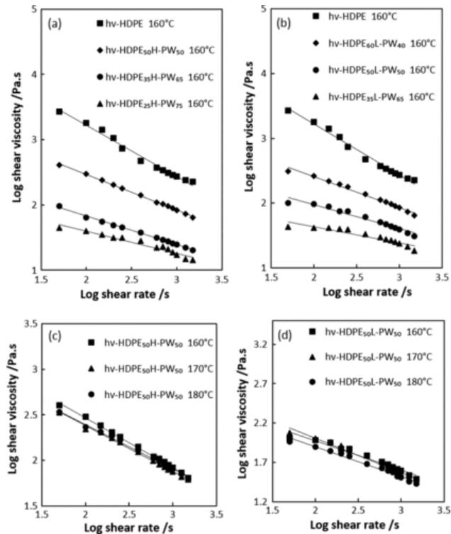
**Fig. 11** Capillary rheology: plots of log shear viscosity versus log shear rate for (a) hv-HDPE and hv-HDPE/H-PW and (b) hv-HDPE and hv-HDPE/L-PW blends at  $160 \text{ }^\circ\text{C}$ ; plots of log shear viscosity versus log shear rate for (c) hv-HDPE<sub>50</sub>H-PW<sub>50</sub> and (d) hv-HDPE<sub>50</sub>L-PW<sub>50</sub> blends at three different temperatures.
