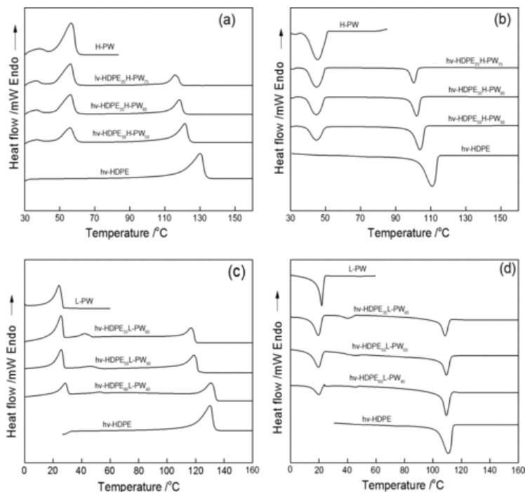
**Fig. 4** DSC thermograms for (a) heating curves of H-PW, hv-HDPE and hv-HDPE/H-PW blends; (b) cooling curves of H-PW, hv-HDPE and hv-HDPE/H-PW blends; (c) heating curves of L-PW, hv-HDPE and hv-HDPE/L-PW blends and (d) cooling curves of L-PW, hv-HDPE and hv-HDPE/L-PW blends.
