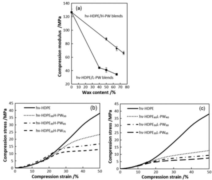
Fig. 10 Compression testing results of (a) variation in compression modulus of hv-HDPE, hv-HDPE/H-PW and hv-HDPE/L-PW blends, as a function of wax content; stress–strain curves for (a) hv-HDPE and hv-HDPE/H-PW blends and (b) hv-HDPE and hv-HDPE/L-PW blends.
