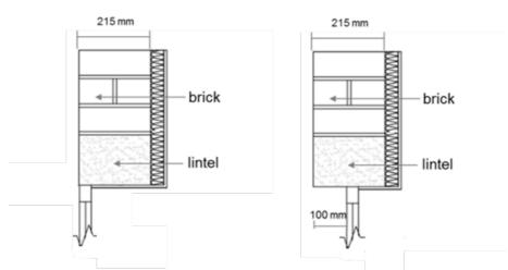
Figure 1 Lintel cross section detail, with window located at 0 mm (left) and 100 mm (right) from the external surface.
