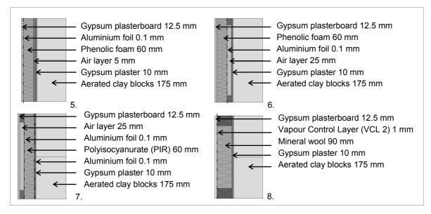
FIG 3. Construction assemblies of the conventional insulation systems, samples 5 to 8
