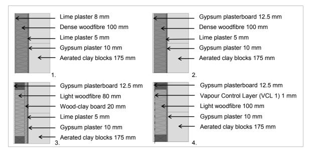
FIG 2. Construction assemblies of the capillary active insulation systems, samples 1 to 4
