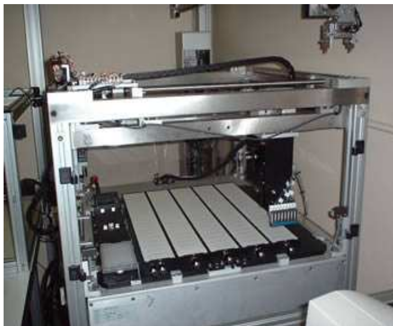
Figure 2.4: The LUSI aspirating-dispensing ink-jet printer, capable of automatically mixing and printing ink samples. The ink wells containing ink supplies are located at the bottom left. Spare wells for mixing are also available. The slides are located in the centre of the picture and are printed using the eight channel print head (centre right). The LUSI gantry gripper is shown at the top-right of the picture.
