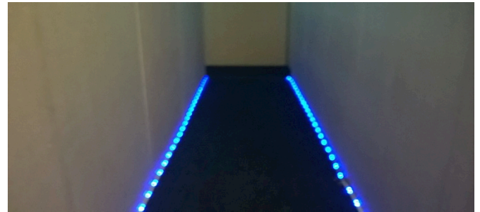
Figure 2. LED lights positioned at floor level of a corridor in order to assess the effect of this visual cue on participant performance.
