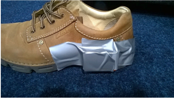
Figure 3. Attachment of the IMU to the heel of the shoe. An alignment jig was placed under the IMU during attachment to keep it horizontal.
