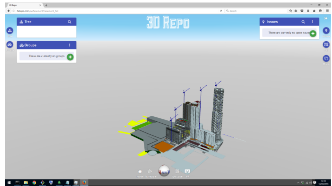
Figure 7: A large 3D scene federated from 19 individual sub-projects consisting of over 1m components and 50m triangles. Each of the buildings and the basement are delivered by different teams of companies using various types of software such as Autodesk Revit, Graphisoft ArchiCad, Tribble Tekla, etc. Left is the 3D Repo GUI desktop application and right the 3drepo.io web app in Firefox. Without support for multipart, this scene would not run in either of the systems. Model courtesy of Canary Wharf Contractors Limited.
