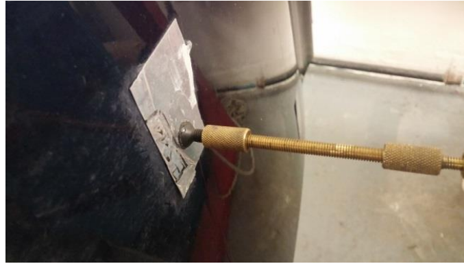
Figure 2.2: Connection method using the stinger and screw. The screw has been fixed onto the vehicle surface using superglue.
