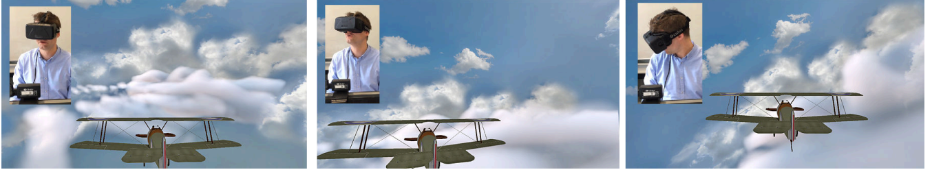
Figure 5: Volumetric novel-view synthesis in a game where the view from an airplane surrounded by moving clouds is controlled by a HMD. The background is sky box, while the foreground clouds are volume-lit and reprojected using our approach from a five-frame latency.
