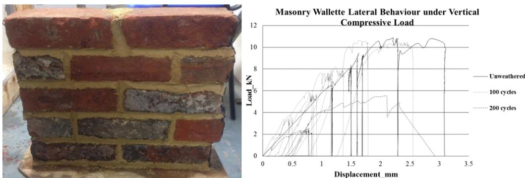
Figure 2: Masonry wallette specimen (left) and comparative assessment of weathered and unweathered masonry wallettes (right)
