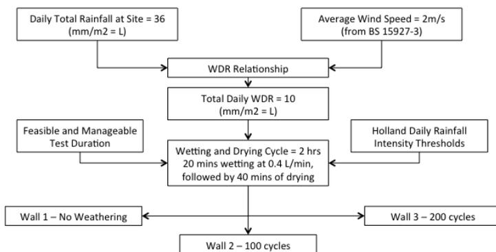
Figure 1: Route map demonstrating weathering sequence design process
