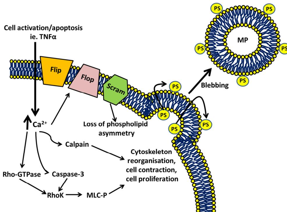
**Figure 1: Schematic of the microparticle formation process**
