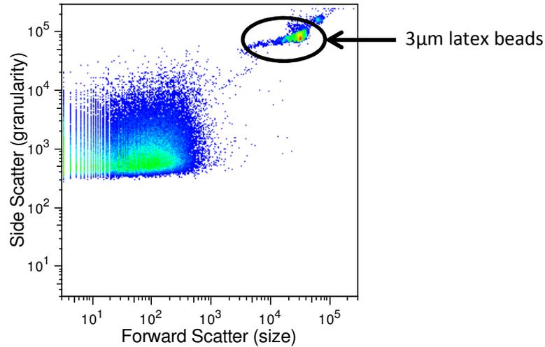
**Figure 8. Detection of 3µm latex beads**
