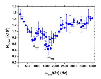
FIG. 6. OCDT radial frequency measurement: number of atoms in the OCDT ( $N_{OCDT}$ ) as a function of the laser intensity modulation frequency ( $\omega_{mod}$ ). Errorbars indicate the standard deviation of the averaged values plotted in the graph.
