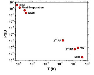
FIG. 8. Evolution of *PSD* as a function of the temperature of the atomic cloud throughout the experimental sequence. Error bars are concealed by the markers representing experimental points.
