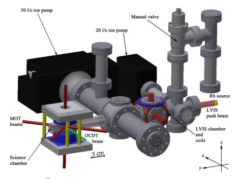
FIG. 1. Sketch of the vacuum chambers for <sup>87</sup>Rb BEC. The Rb solid reservoir is contained at the bottom of the blind flange on the right hand side. LVIS and MOT main coils are highlighted in blue; respective laser beams are indicated in red. Green labels the optical dipole trap beam. For the sake of simplicity, only one beam of the optical crossed dipole trap is shown.
