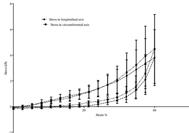
Fig 2: Stress-Strain graph for oesophageal specimens showing mean (kPa) and standard deviation
