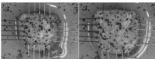
Fig. 1: Images of oesophageal sample loaded on CellScale biaxial testing system at 0% strain (Left) and maximum strain (Right).
