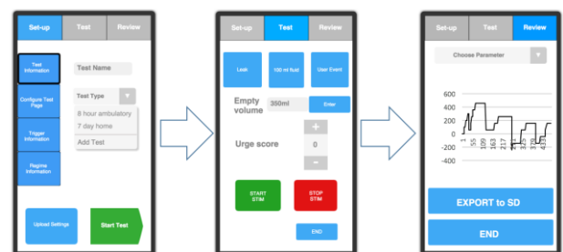
Figure 1. Initial designs for User Interface. From left to right - 1. Parameter and information input 2. Patient diary and control interface 3. Review and export window
