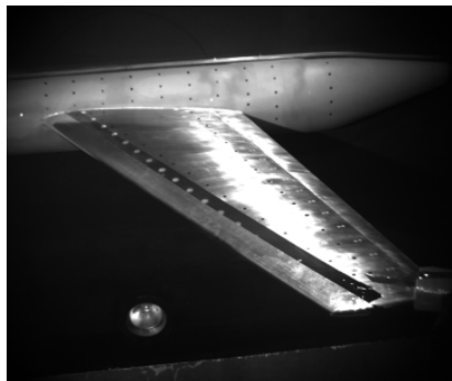
Figure 1. Example of the impact of ambient lighting on measurement of passive wing targets in a wind tunnel.
