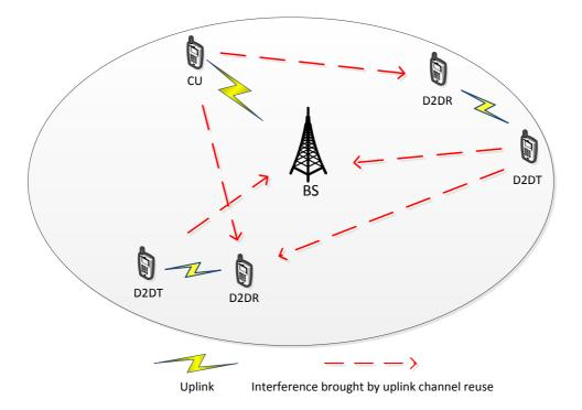
Fig. 1. The model of D2D communications underlaying a cellular network in the uplink.
