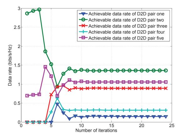
Fig. 6. The convergence behavior for the rates of the D2D pairs using (decentralized) Algorithm 3.
