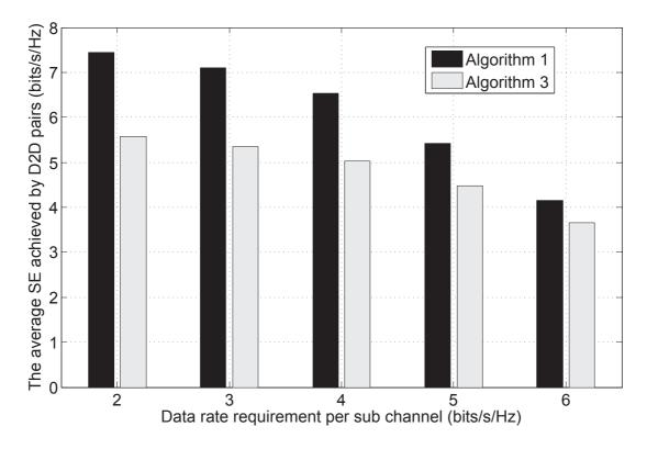
Fig. 2. The spectrum efficiency results for the D2D pairs against the rate requirements of the CUs.
