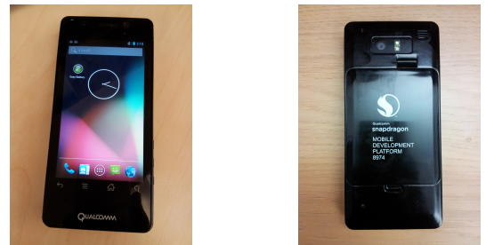
Figure 9: Snapdragon 800 Mobile Development Platform for Smartphones used for the DeepEar prototype development.
