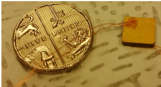
Figure 7.2: Image of a miniature ceramic piezoelectric transducer to be embedded on a microfluidic device. Copper wire was connected to the transducer with the conductive adhesive gel.
