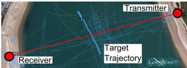
Fig. 4. GPS track showing target trajectory for first described experimental data.
