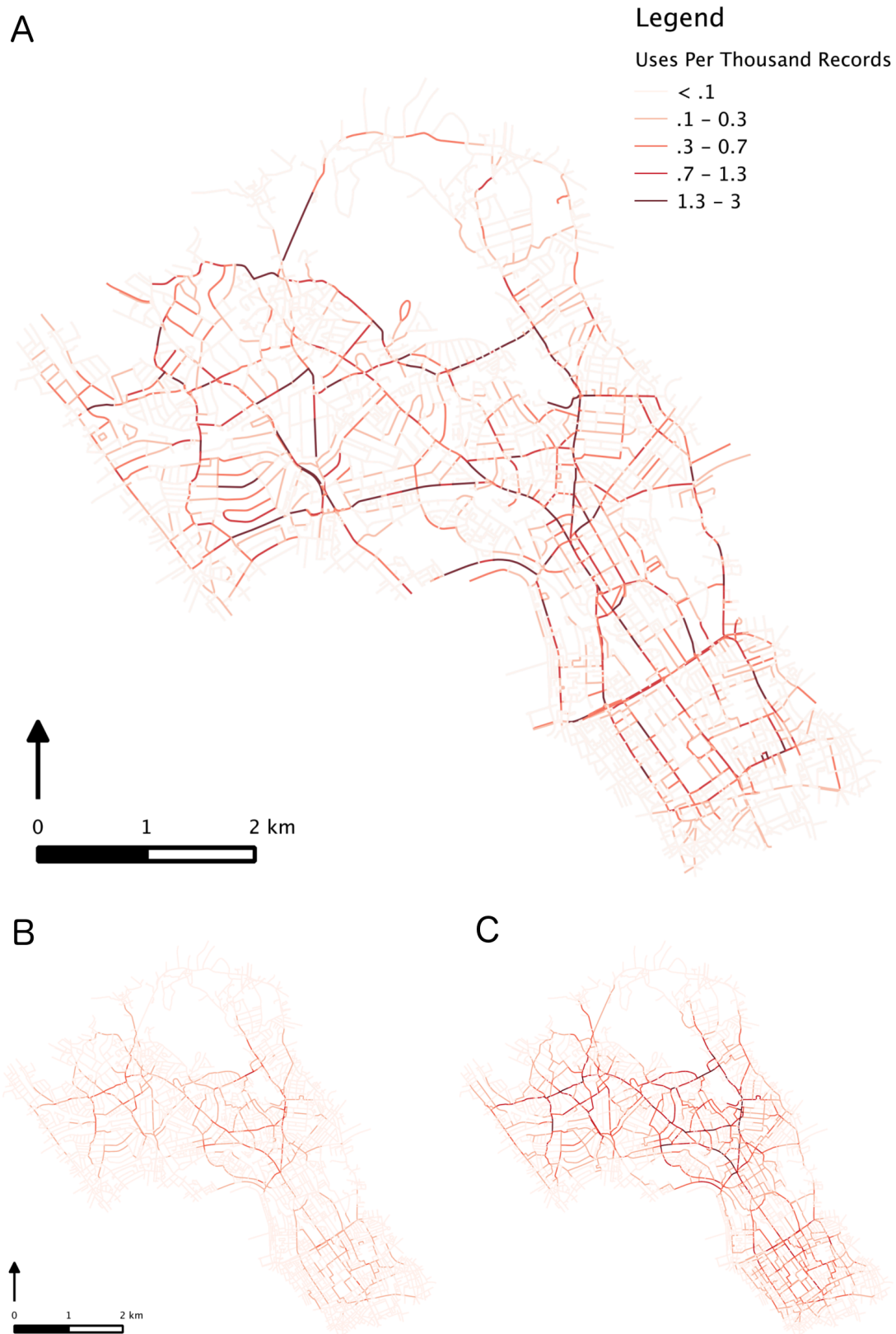
Figure 1. Normalised heatmaps showing the road usage associated with the real data (A), the random-patrolling model (B), and the tasking-service model (C).
