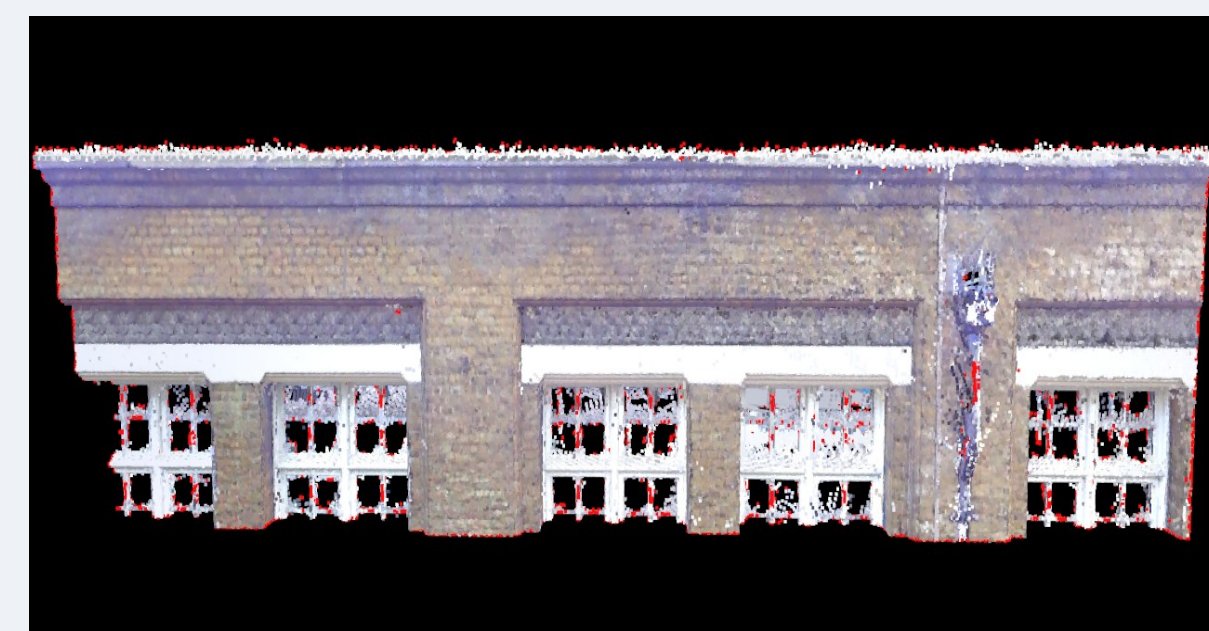
Figure6 Boundary of wall and windows
