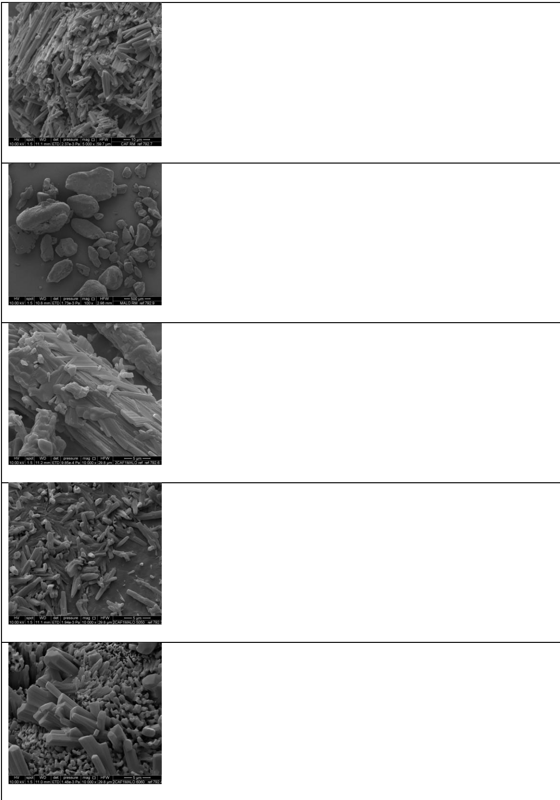
Figure 8. SEM images of (from top to bottom) CAF, MAL, the reference co-crystal, S50:P50 and S60:P60.
