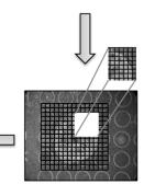
4. At each position an MS spectrum along with its image coordinates is acquired
