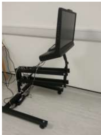
Figure 1 Picture of the TX-300 Tobii Eye Tracker attached to the height adjustable arm
