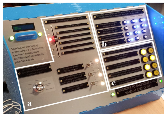
Figure 2. An example question box with different controllers: toggles, slider, rotary dial; check buttons and yes/no buttons.
